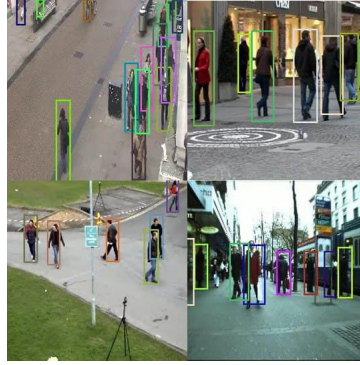
Fig. 14. Visual example of detection and tracking pipeline's output.
