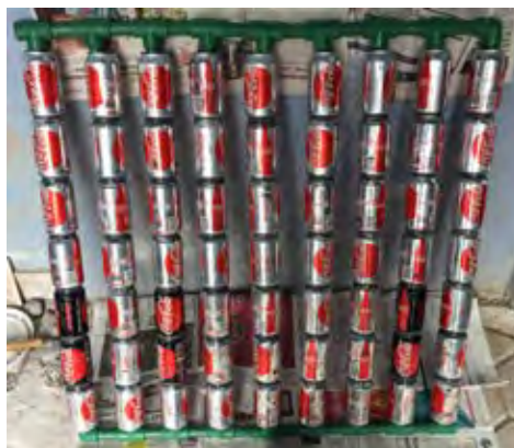
Figure 2. Columns of aluminum cans and Tuboplus connections
