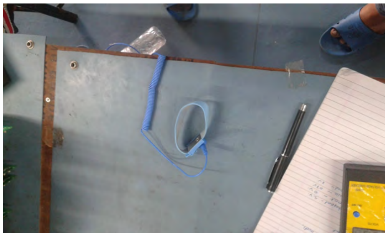
Figure 5. ESD Wrist straps usedat D.C.P.L
