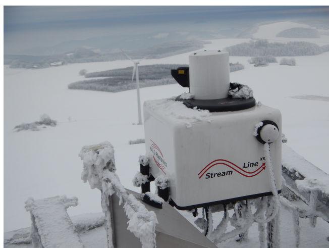
Figure 1: Scanning wind lidars allow wind speed and direction to be measured from up to 10 km away. Image courtesy of Stuttgart Wind Energy, University of Stuttgart.
