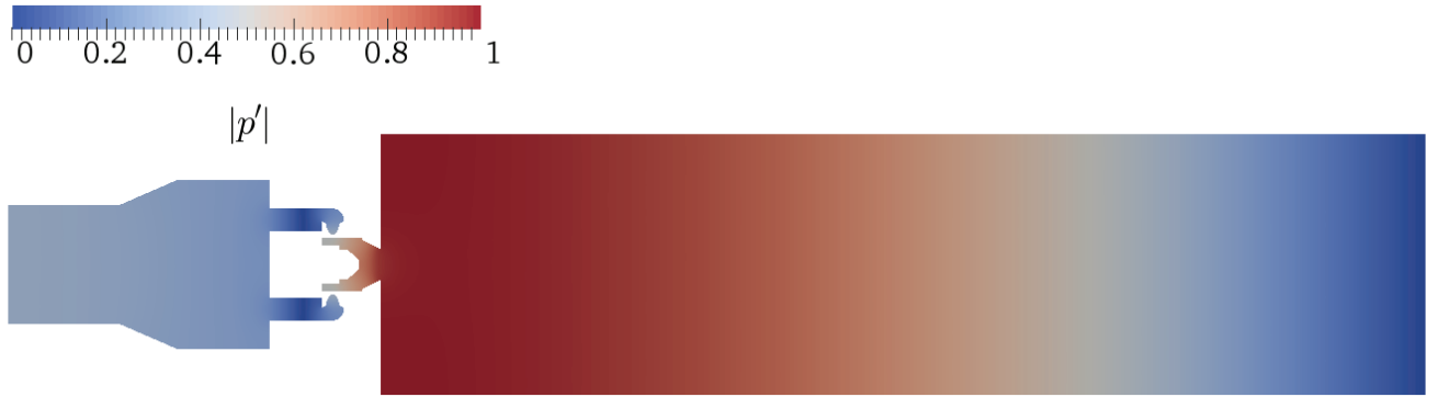
Figure 15: Acoustic mode obtained with Helmholtz solver.
