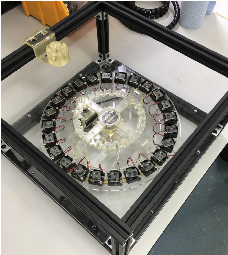
Figure 20 Stirring ring and Driven wheel added. A magnet mount base is glued to each fan.
