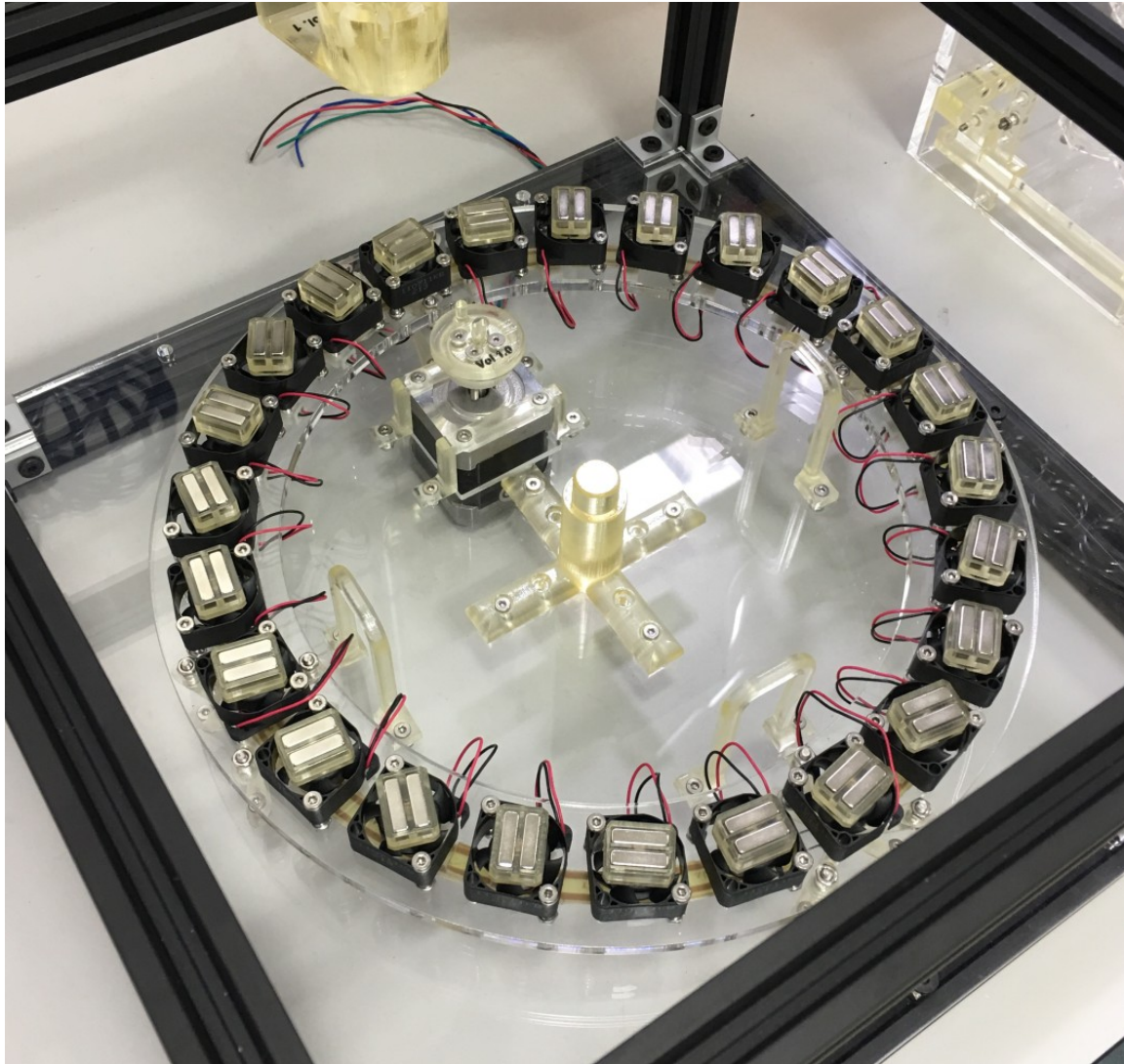
Figure 24 Magnets secured in the housings are added to the base mounts on the stirring ring
