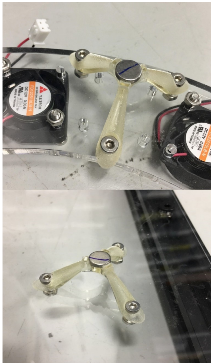
Figure 17 Stirring ring tripod magnets marked for alignment, glue to the tripod 3D prints
