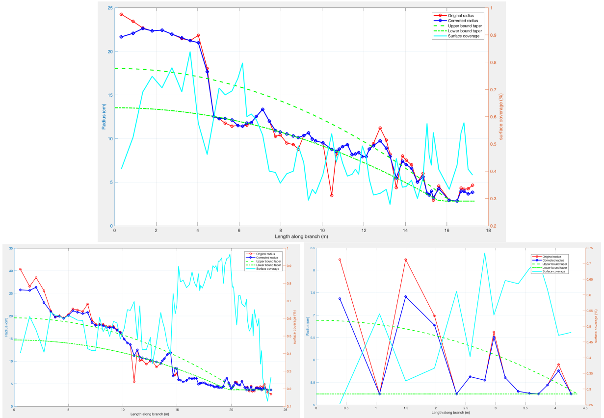
Figure 21: Cylinder radius modification with parabolas. Red circles and lines denote the original fitted radius, green lines denote the maximum and minimum radius parabolas, blue circles and lines denote the final modified radii, and the light blue lines denote the surface coverage (right vertical axis).
