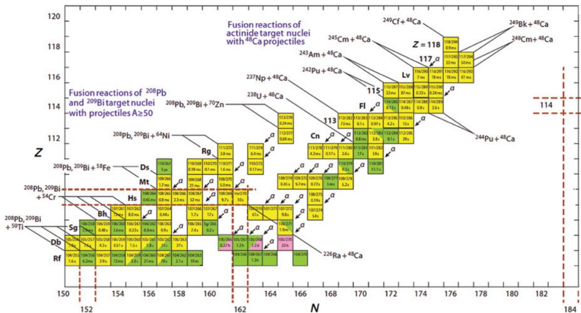
**Fig. 1:** Map of the region of superheavy nuclei relevant to this report including the reactions used to synthesize the various nuclides. (Adapted from [7].) The colors indicate different decay modes for nuclide  $Z/A$  along with its half life in milliseconds (ms), seconds (s), minutes (m) or hours (h) following the convention and data of [7],  $q, v$ .
