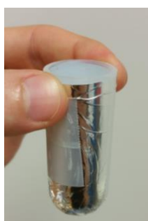
Fig. 1. 30 mL FEP vial with Al foil to mitigate electrostatic charging.
