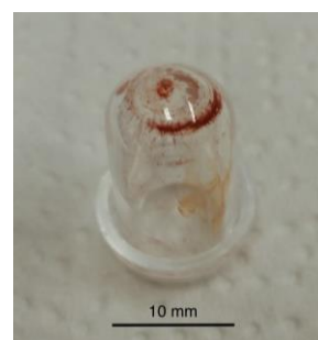
Fig. 3. Quartz crucible after sample transfer turned upside down, illustrating transfer losses.
