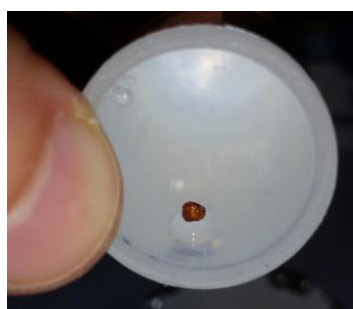
Fig. 2. Transfer of the Fe-carrier pellet using a 50-100 \mu\text{L} droplet.
