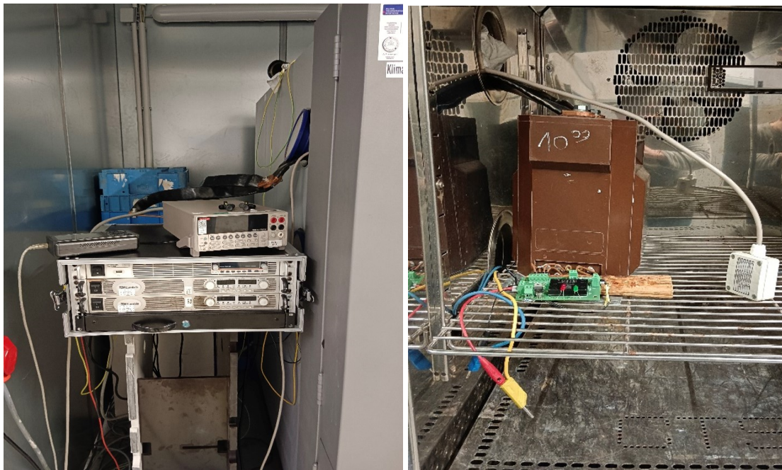
Figure 26: Temperature compensation setup (left); Hall sensor in the environmental test chamber (right).
