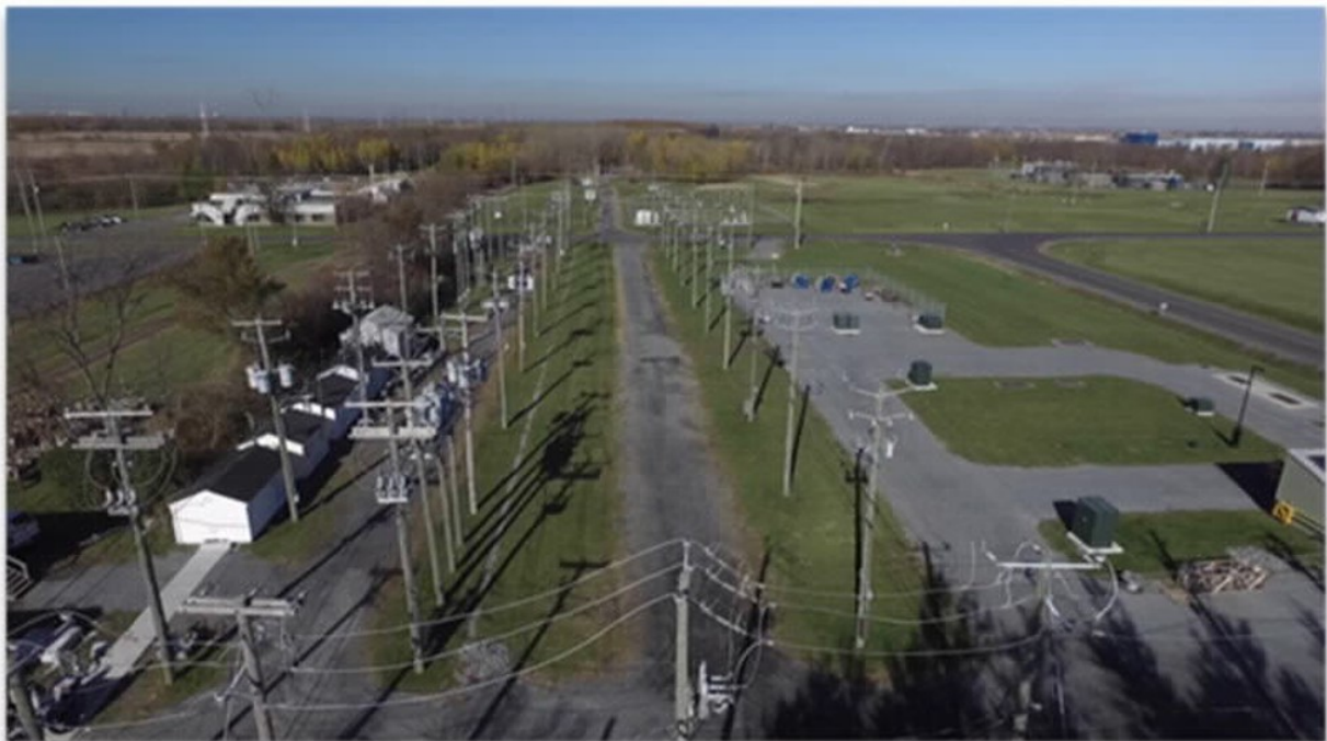
Figure 53: Full-scale distribution test line test setup at IREQ (source: Hydro-Québec).
