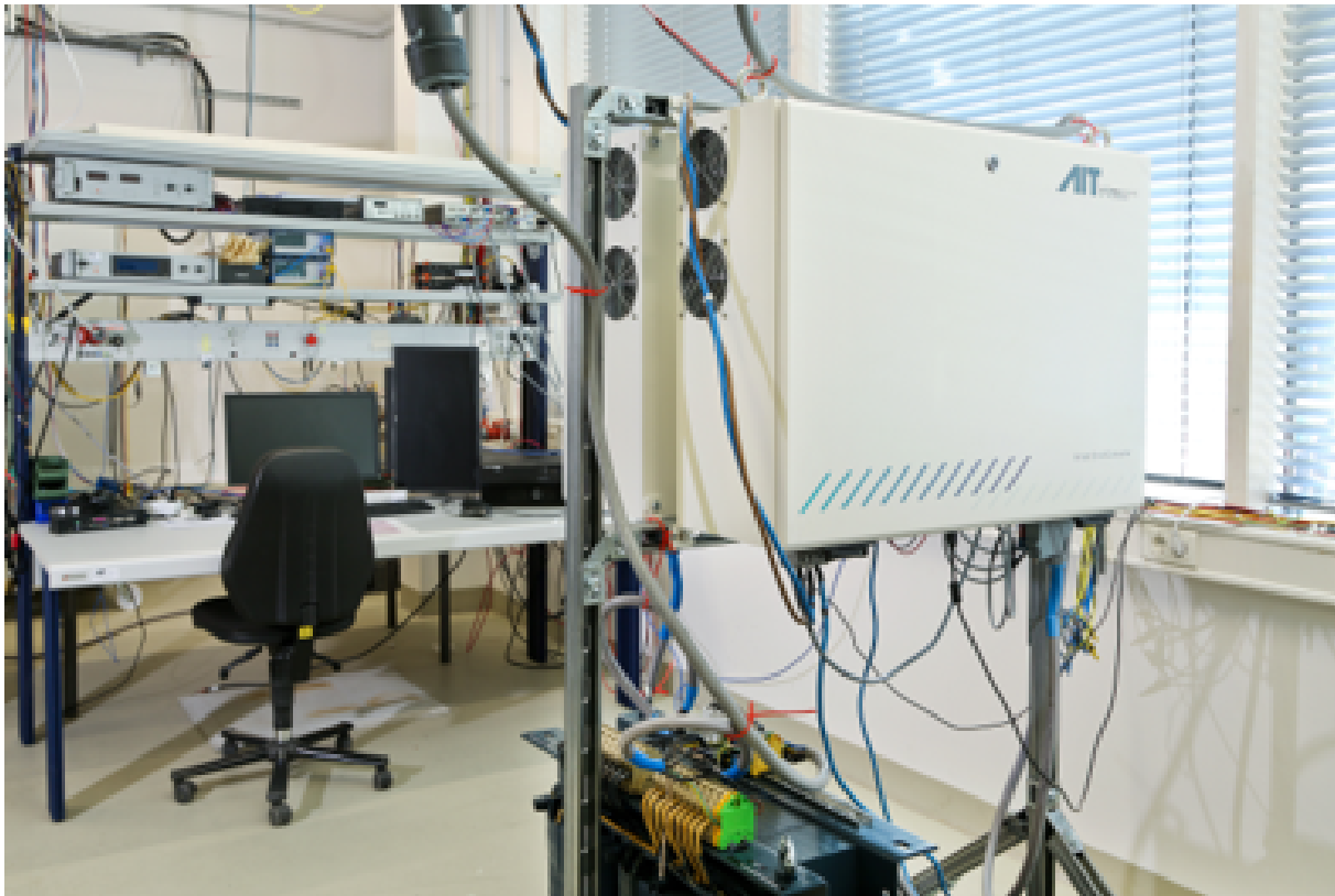
Figure 10: Laboratory setup with two AIT smart grid converters in a back-to-back setup.
