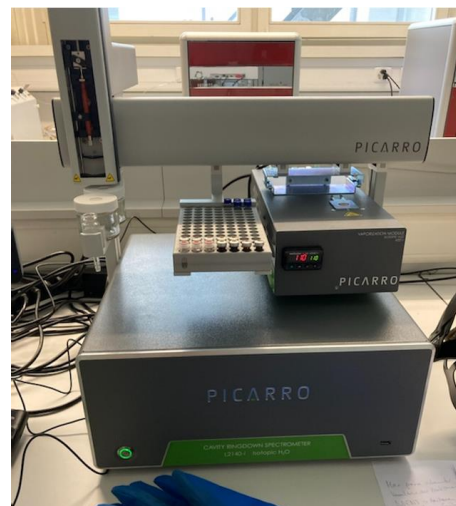
Figure 11: Cavity Ring Down Spectrometer (CRDS) used at the lab of the Institute of Geography at the University of Berne
