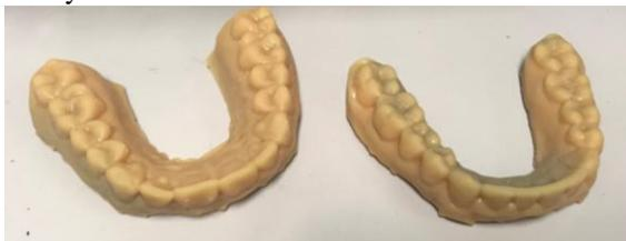
**Figure 1. Dental mold produced by Fused Deposition Modelling method**
