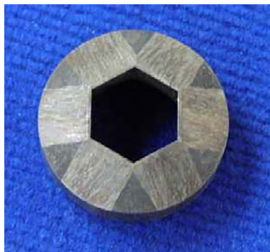
Fig. 10.3 Appearance of hardened blanking die
