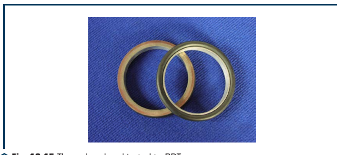
○ Fig. 10.15 The end seals subjected to PDT
