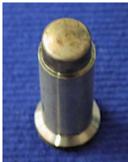
Fig. 10.6 Hardened punch for hot forming of metal
