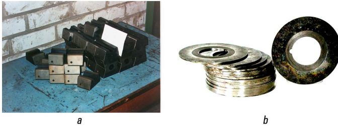
Fig. 10.1 Hardened knives for cutting rolled stock: a – steel sheets; b – sections
