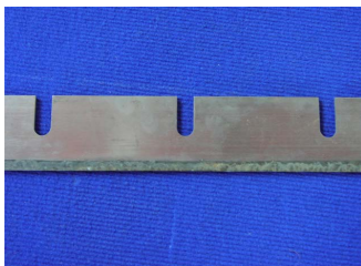
○ Fig. 10.9 Hardened knife for wood crushing
