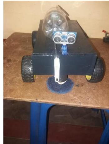
Fig 4. Final prototype of floor cleaning robot
