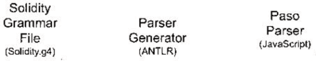
Figure 3.1: The Parser Generator takes a file containing the Solidity grammar rules. It produces a PASO Parser, i.e. a parser in JavaScript computer language that can be run in a client browser.
