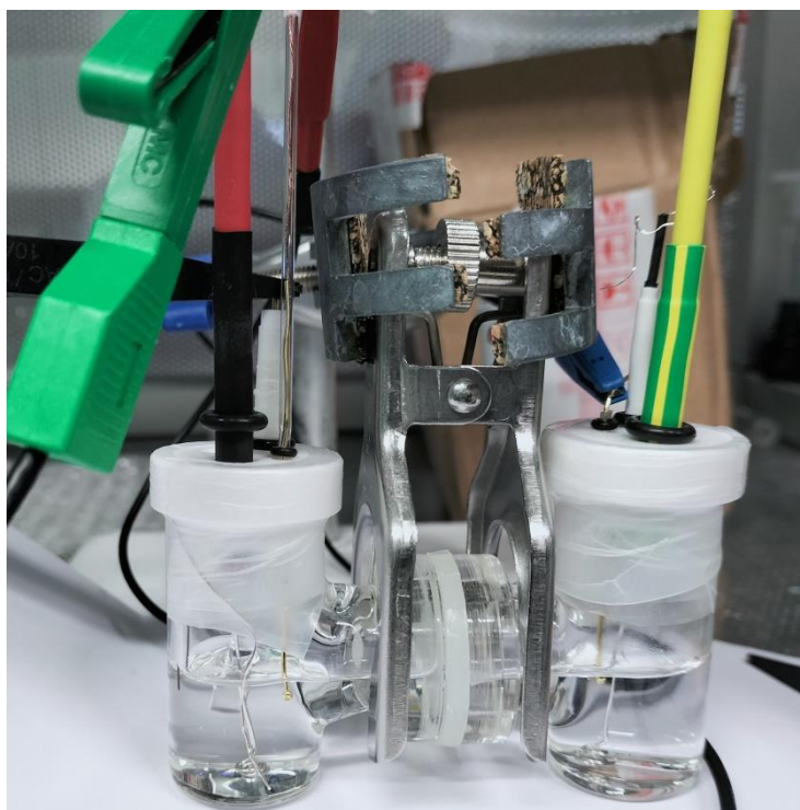
Fig. S2. Image of the 4-electrode closed bipolar electrochemical cell (CBPEC) used in this study. An H-type electrochemical cell was adapted to perform bipolar electrochemistry under aerobic and anaerobic conditions. An impermeable silicone rubber sheet separated the aqueous and organic compartments. Each pole of the bipolar electrode consisted of a polycrystalline gold electrode, with one immersed in each compartment, denoted P_w in the aqueous phase and P_o in the organic phase, and connected with an electric wire. The composition of the 4-electrode CBPEC configurations used are described in Scheme 2.
