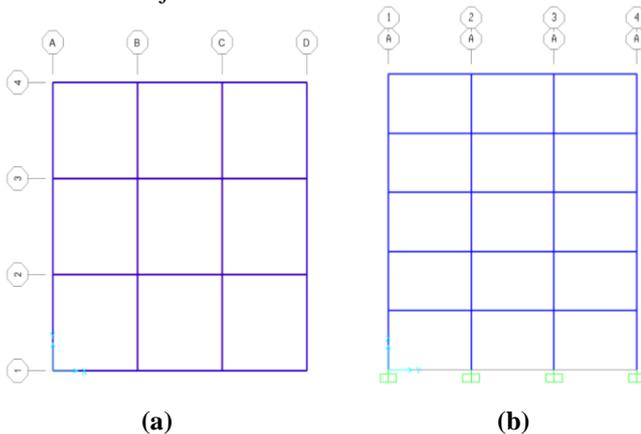
**Figure; 2 (a ) Plan and (b) Elevation of 3 bay, 5story building**
