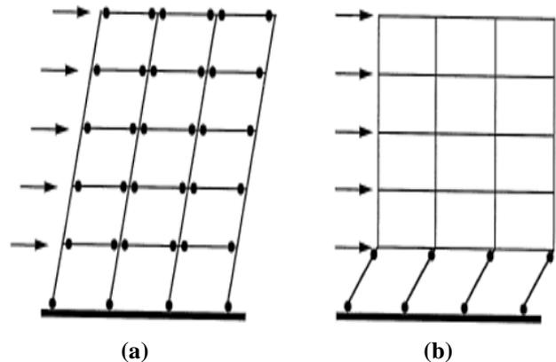
**Figure1: (a) Mechanisms of Strong Column Weak Beam and (b) Weak Column Strong Beam [7]**
