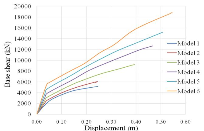
**Figure: 3 Displacement versus base shear curve**
