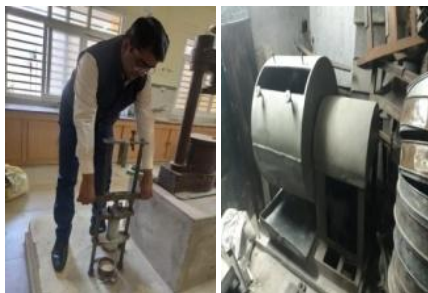
Fig. 3: Laboratory setup and Equipments for AIV and LAAV tests (IS: 2386-Part 4)
