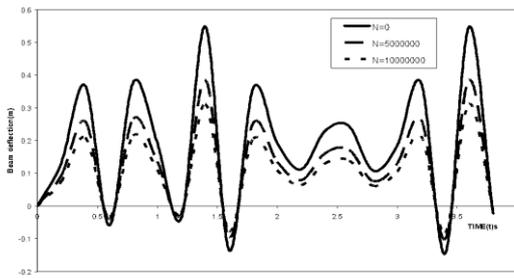
**Figure 6. Displacement response of beam (harmonic magnitude) for fixed FM=4000000, Ro =0.5 and various values of N.**
