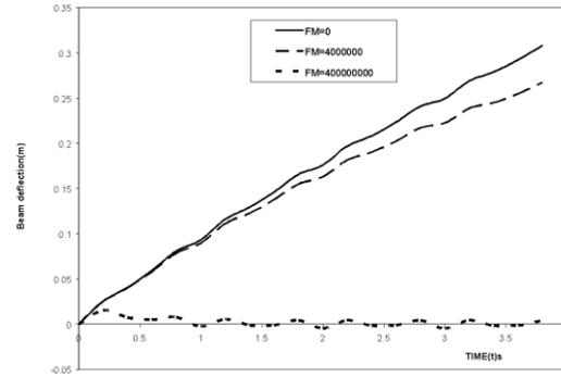
**Fig. 2. Deflection of beam (constant magnitude) for fixed  $R_0=0.5$ ,  $N=500000$  and various values of FM.**
