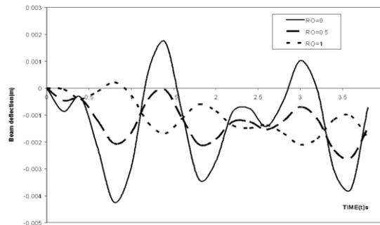
**Figure 4. Displacement response of beam (harmonic magnitude) for fixed  $\text{FM}=4000000$ ,  $N=500000$  and various values of  $R_0$ .**
