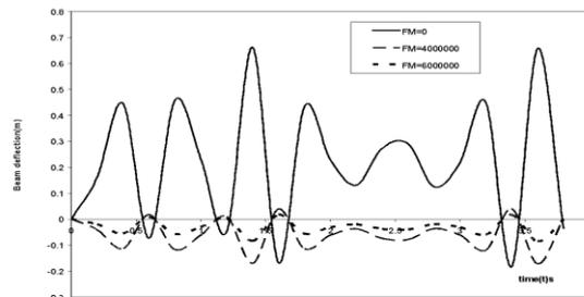
**Figure 5. Displacement response of beam (harmonic magnitude) for fixed  $R_0=0.5$ ,  $N=500000$  and various values of FM.**
