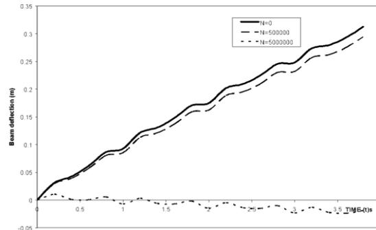
**Fig. 3. Deflection of beam (constant magnitude) for fixed  $R_0=0.5$ ,  $\text{FM}=4000000$  and various values of N**
