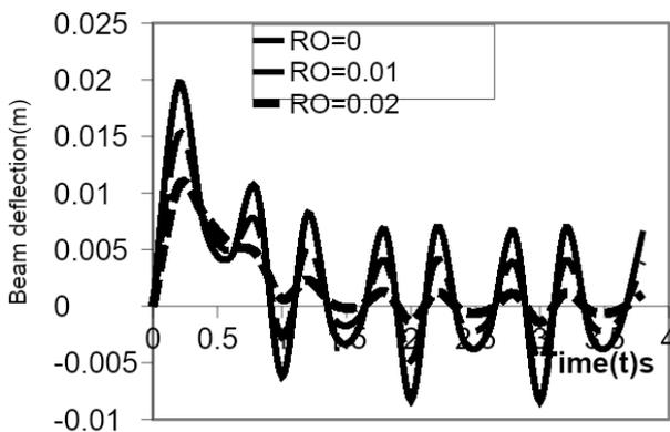
**Fig. 1. Deflection of beam (constant magnitude) for fixed  $\text{FM}=4000000$ ,  $N=500000$  and various values of  $R_0$ .**
