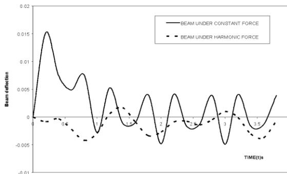
**Figure 7. Comparison deflection of the beam on exponentially decaying foundation for constant and harmonic magnitude.**
