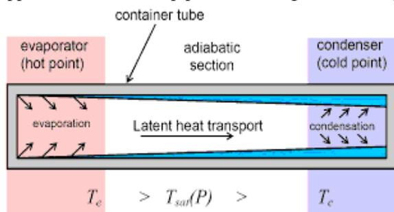
Fig.1.1.Heat pipe structure
