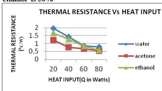
**Fig.3.1.variation of thermal resistance of water, acetone, ethanol**
