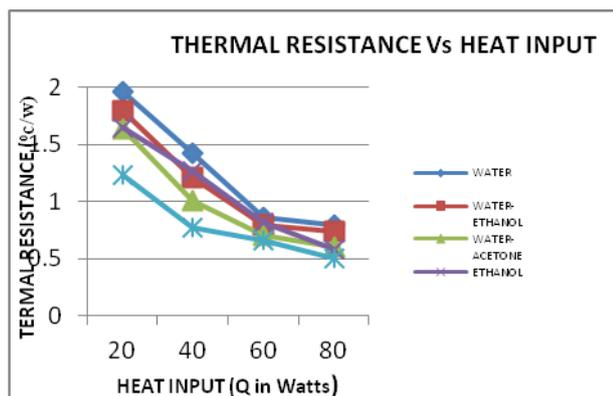
Fig.3.9.comparison between thermal resistance of water, acetone, ethanol, water-ethanol mixture, and water-acetone mixture.
