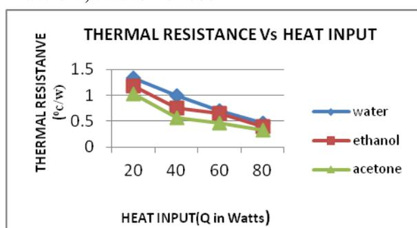
**Fig.3.2.variation of thermal resistance of water, acetone, ethanol**
