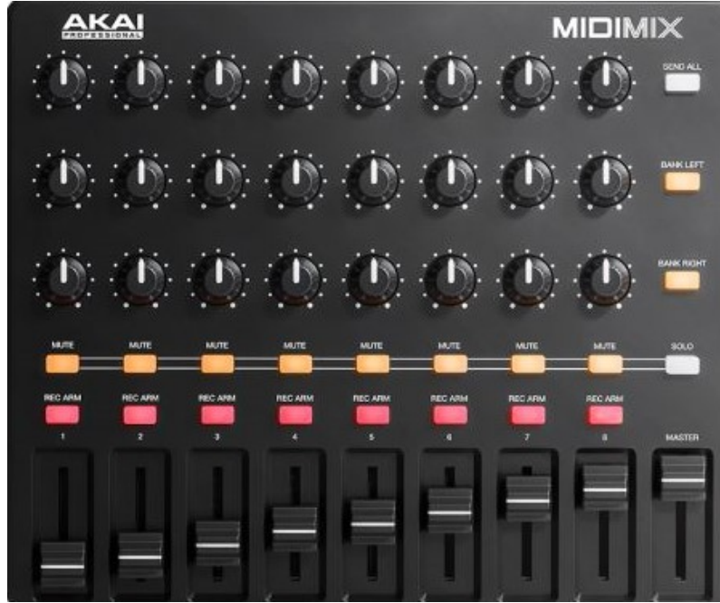
Figure 8: The AKAI MIDIMIX MIDI controller. Each fader and red button is linked to one stimuli, where the button changes the stimulus playback and the fader serves to mark it ( C in Figure 9). The vertical array of buttons in the right side is used to stop the playback, play the reference stimulus and to pass from one group to the next one ( B in Figure 9). Stickers were added during the tests to help the subjects.
