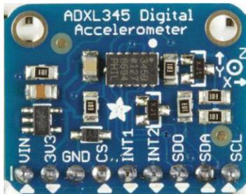
Fig. 3. Accelerometer (ADXL345)
