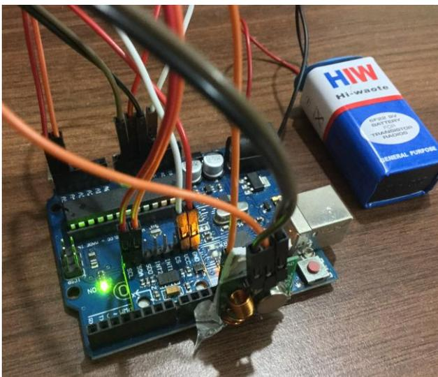
Fig. 6. Transmitting module.
