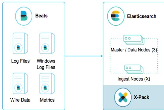
**Fig 4: Shows inside details of an Elasticsearch cluster**
