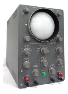
Figure 1: Heathkit oscilloscope model O-12 with 5-inch tube, ca. 1958. Photo by the author. Licensed under CC BY-NC-SA 4.0.
