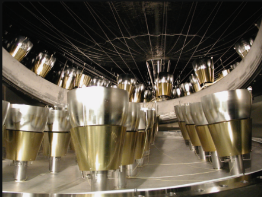
Internal view of the Borexino liquid scintillator containment liquid scintillator vessel. From the photo several parts of the detector are visible: the photomultipliers (silver-like color) the mu-metal shielding (brass-like color) the bottom of the outer nylon vessel (upper part of the photo).
