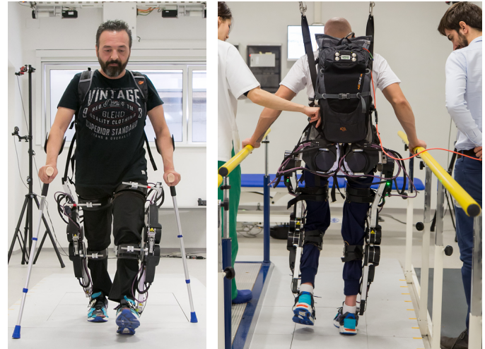
Fig. 1: SCI test pilots using the modular exoskeleton in knee-ankle configuration (KA) on the left and hip-knee-ankle configuration (HKA) on the right.
