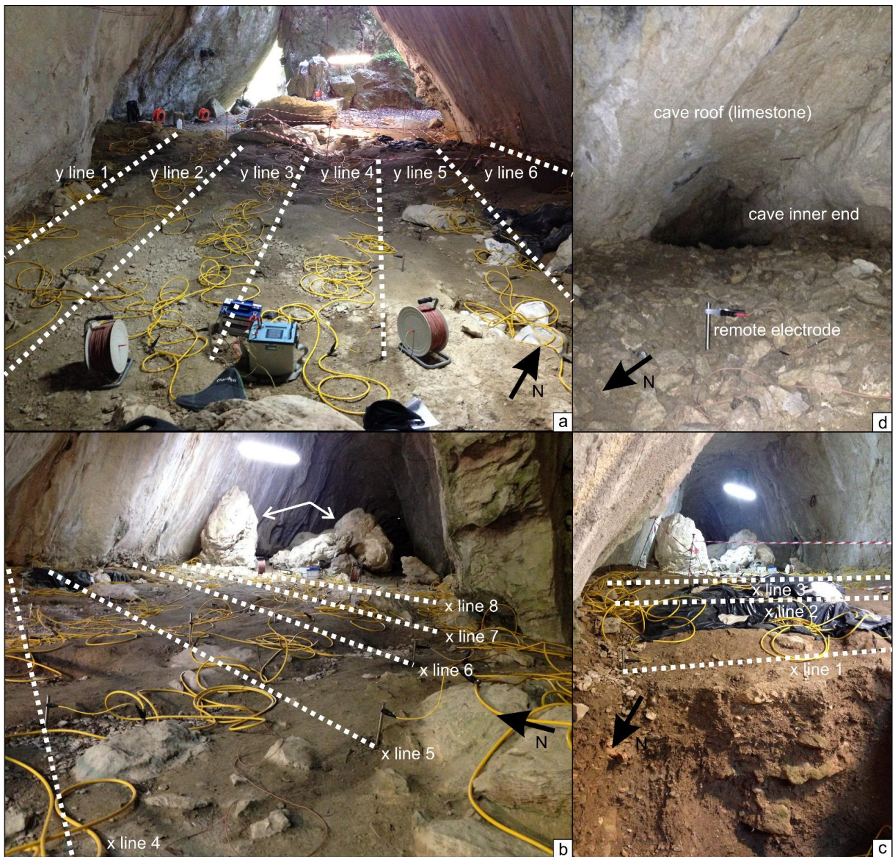
Fig. 2: pictures showing different views of the ERT survey grid.
