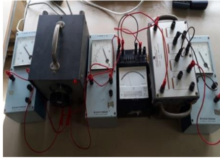
Figure 8. Practical connection of transformer short-circuit test
