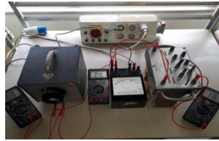
Figure 6. Practical connection of transformer open-circuit test
