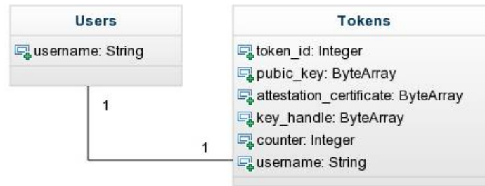
Figure 4-8: Database Schema of the project
