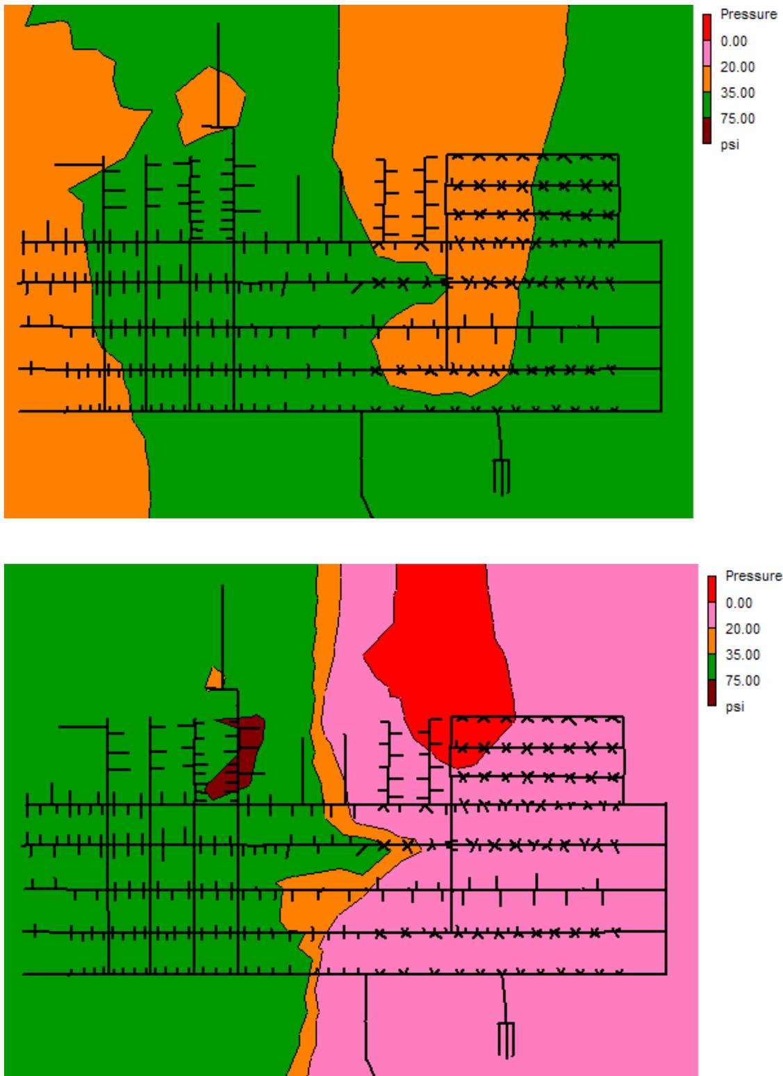
Figure 3. Maps of system static pressure under 500 gpm fire flow at HY44 with main MA802 open (top) and closed (bottom).
