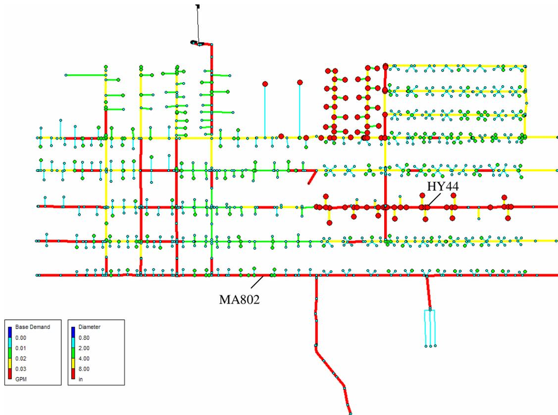
Figure 2. Micropolis water distribution system as modeled in EPANet.
