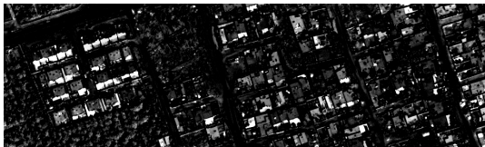
Filter by rec. f - \gamma_R^B(f) ( B : disk radius 7 pixels)
