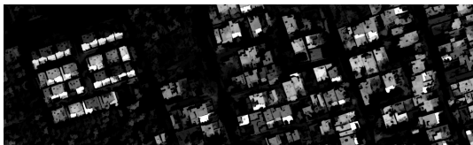
Attribute filter \gamma^T(f) with T = (R > 0.3) \wedge (I < 0.5) \wedge (50 < A < 5000)
