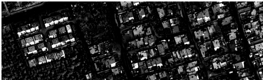
Filter by rec. f - \gamma_R^B(f) ( B : disk radius 11 pixels)
