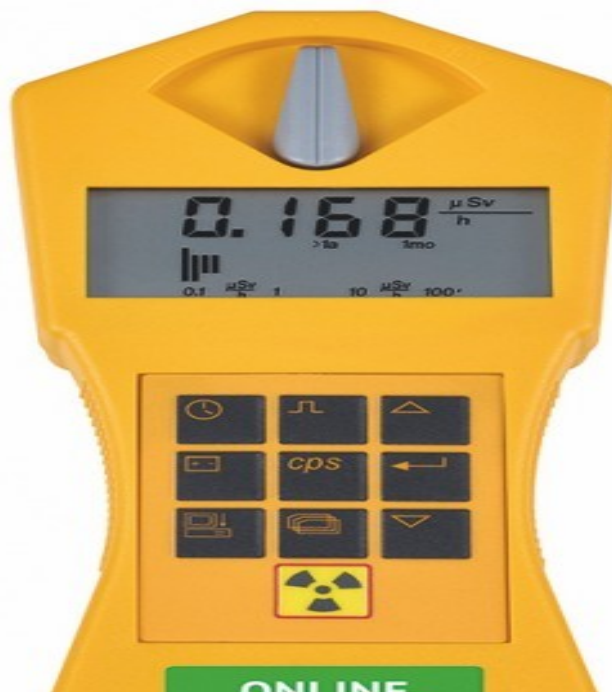
Figure 1. The gamma radiation detector Gamma Scout Online
