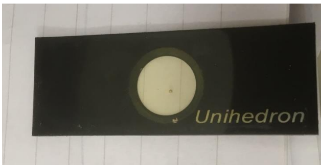
Figure 9 Browning of the transparent cover of one of the SQM's
