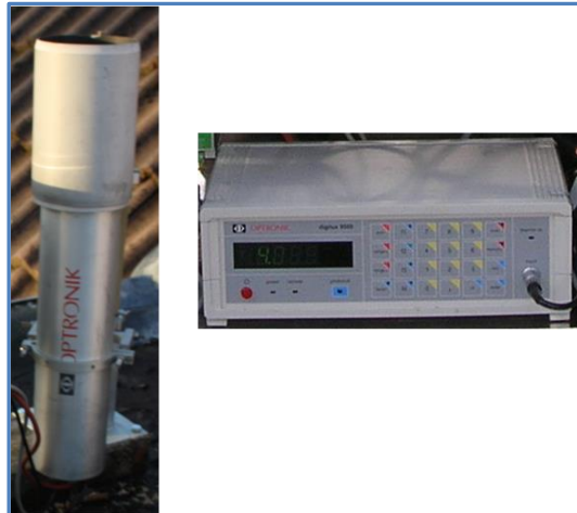
Figure 5 The Digilum. Left: the measuring head. At the right the read out unit.
