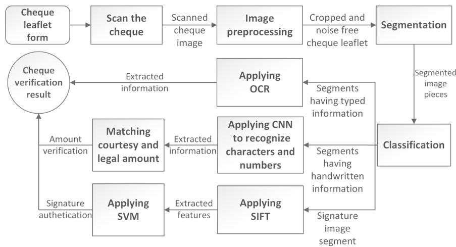
Fig. 5 Block diagram of bank cheque verification process
