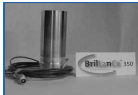
Thin BrillanCe plates Coupled to fast PMTs
