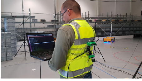
Figure 6. Human operator wearing the Safety Vest equipped with vision sensor for localization.
