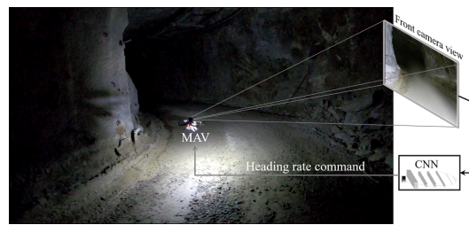
Fig. 1: The proposed approach for classifying the images from the forward looking camera during autonomous navigation in underground mines. Supplementary Video: https://youtu.be/j3N8ij9MfSA .
