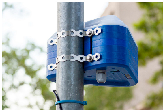
Fig. 33. Smart Citizen Station V1.0 outdoor installation.
