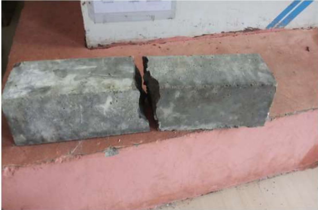
Fig 11 : Crack Pattern of Beams
