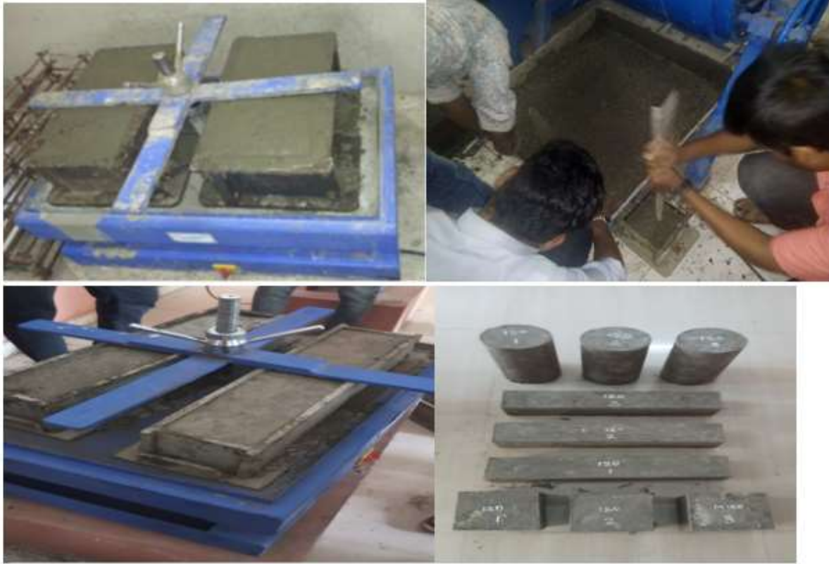
Fig 5 : Compaction of Concrete
