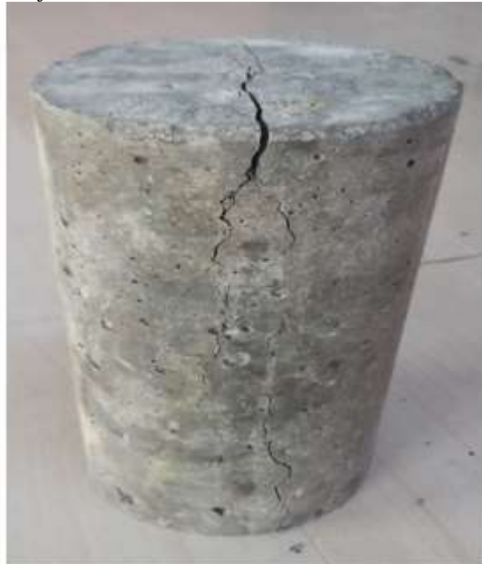
Fig 10 : Crack Pattern of Cylinders
