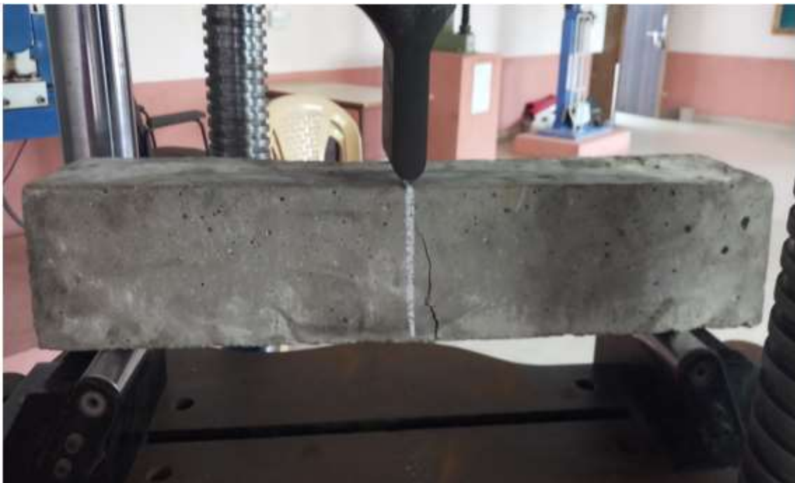
Fig 12 : Crack Pattern of Beams
