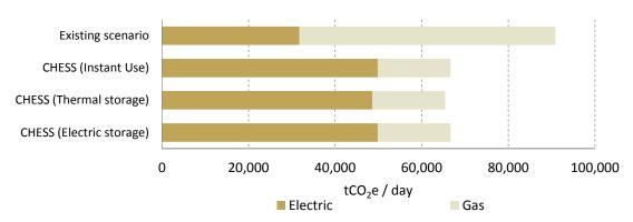
Figure 85. Dwellings totals equivalent CO2 emissions in the existing scenario and each CHESS Setup configurations
