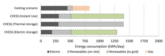
Figure 22. Dwellings totals energy uses/consumption in the existing scenario and each CHESS Setup configurations
