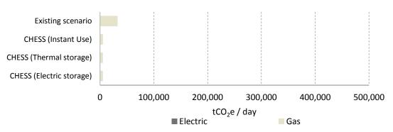
Figure 56. Dwellings totals equivalent CO2 emissions in the existing scenario and each CHESS Setup configurations
