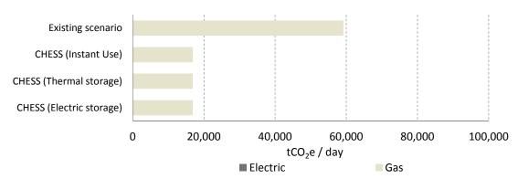
Figure 95. Dwellings totals equivalent CO2 emissions in the existing scenario and each CHESS Setup configurations
