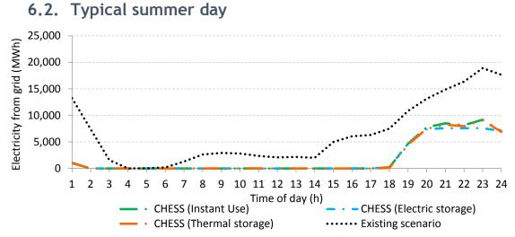
Figure 62. Dwellings existing scenario and CHESS Setup configurations hourly electric grid consumption
