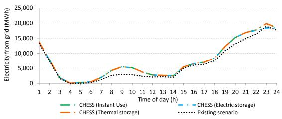
Figure 31. Dwellings existing scenario and CHESS Setup configurations hourly electric grid consumption
