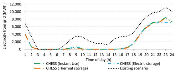
Figure 96. Dwellings existing scenario and CHESS Setup configurations hourly electric grid consumption
