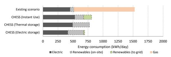
Figure 17. Dwellings totals energy uses/consumption in the existing scenario and each CHESS Setup configurations
