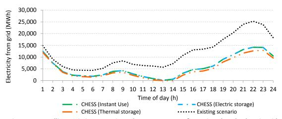
Figure 91. Dwellings existing scenario and CHESS Setup configurations hourly electric grid consumption
