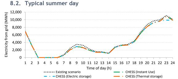
Figure 86. Dwellings existing scenario and CHESS Setup configurations hourly electric grid consumption
