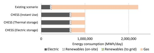
Figure 40. Dwellings totals energy uses/consumption in the existing scenario and each CHESS Setup configurations
