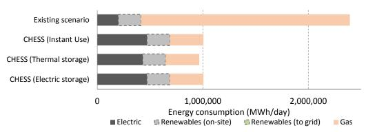
Figure 60. Dwellings totals energy uses/consumption in the existing scenario and each CHESS Setup configurations
