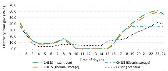
Figure 15. Dwellings existing scenario and CHESS Setup configurations hourly electric grid consumption
