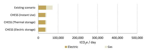
Figure 35. Dwellings totals equivalent CO2 emissions in the existing scenario and each CHESS Setup configurations
