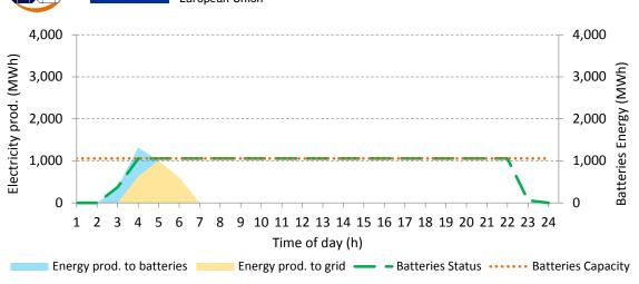
Figure 87. PVs electric production usage and batteries status.
