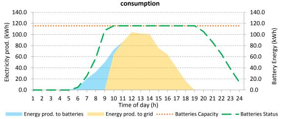
Figure 10. PVs electric production usage and batteries status.
