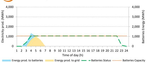
Figure 76. PVs electric production usage and batteries status.
