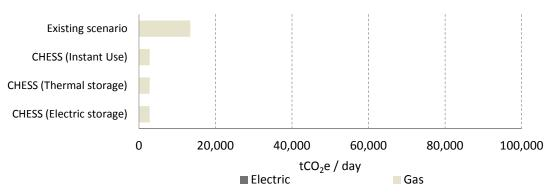
Figure 100. Dwellings totals equivalent CO2 emissions in the existing scenario and each CHESS Setup configurations
