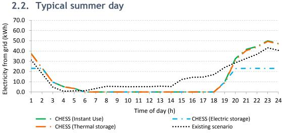
Figure 19. Dwellings existing scenario and CHESS Setup configurations hourly electric grid consumption
