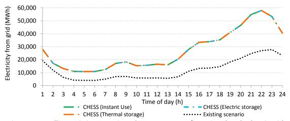
Figure 37. Dwellings existing scenario and CHESS Setup configurations hourly electric grid consumption
