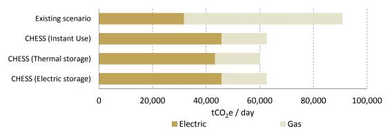
Figure 72. Dwellings totals equivalent CO2 emissions in the existing scenario and each CHESS Setup configurations
