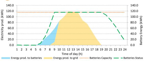
Figure 20. PVs electric production usage and batteries status.
