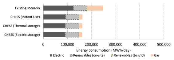
Figure 89. Dwellings totals energy uses/consumption in the existing scenario and each CHESS Setup configurations
