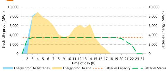
Figure 53. PVs electric production usage and batteries status.
