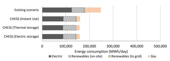
Figure 78. Dwellings totals energy uses/consumption in the existing scenario and each CHESS Setup configurations
