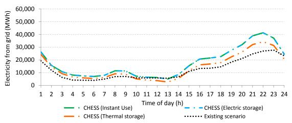
Figure 47. Dwellings existing scenario and CHESS Setup configurations hourly electric grid consumption
