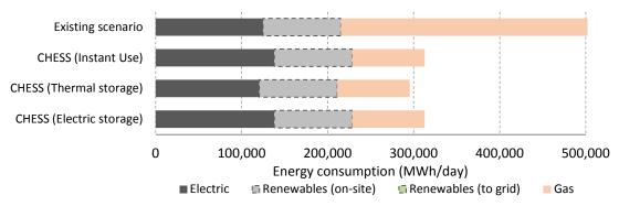
Figure 94. Dwellings totals energy uses/consumption in the existing scenario and each CHESS Setup configurations
