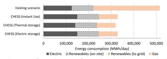
Figure 104. Dwellings totals energy uses/consumption in the existing scenario and each **CHESS Setup configurations**
