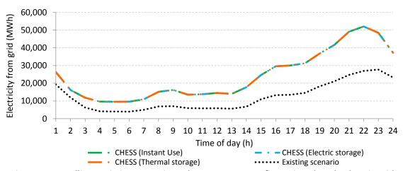
Figure 24. Dwellings existing scenario and CHESS Setup configurations hourly electric grid consumption
