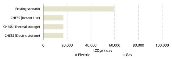
Figure 105. Dwellings totals equivalent CO2 emissions in the existing scenario and each **CHESS Setup configurations**
