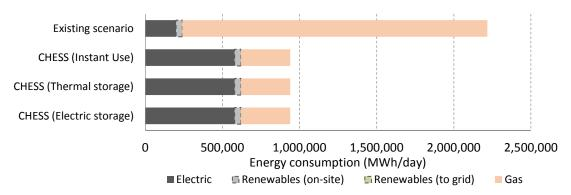
Figure 28. Dwellings totals energy uses/consumption in the existing scenario and each CHESS Setup configurations
