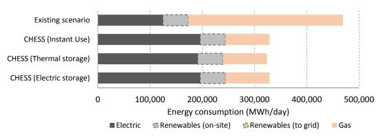
Figure 84. Dwellings totals energy uses/consumption in the existing scenario and each CHESS Setup configurations
