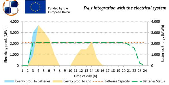
Figure 107. PVs electric production usage and batteries status.
