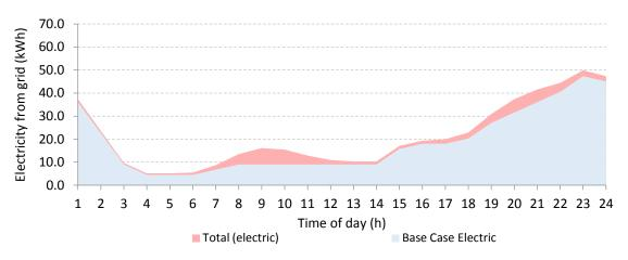
Figure 8. Base Case and Total hourly electric consumption from electrical grid
