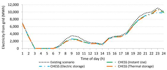
Figure 74. Dwellings existing scenario and CHESS Setup configurations hourly electric grid consumption
