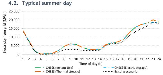
Figure 42. Dwellings existing scenario and CHESS Setup configurations hourly electric grid consumption
