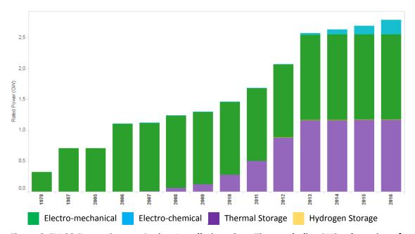
Figure 6. EU-28 Energy Storage Project Installations Over Time excluding PHS, adaptation of DOE database (DOE, Office of Electricity Delivery & Energy, 2016)
