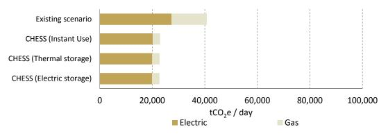
Figure 90. Dwellings totals equivalent CO2 emissions in the existing scenario and each CHESS Setup configurations
