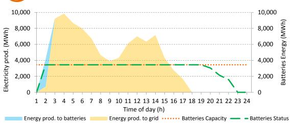
Figure 63. PVs electric production usage and batteries status.
