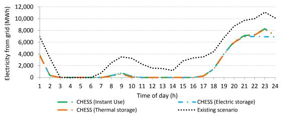
Figure 106. Dwellings existing scenario and CHESS Setup configurations hourly electric grid consumption
