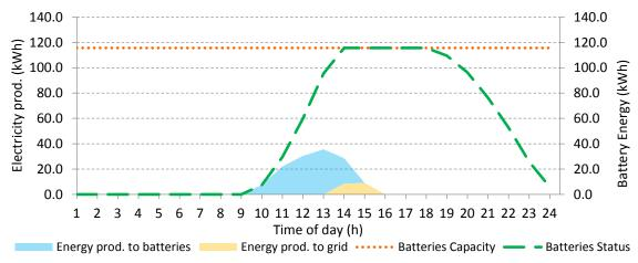
Figure 16. PVs electric production usage and batteries status.
