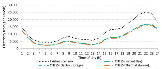
Figure 67. Dwellings existing scenario and CHESS Setup configurations hourly electric grid consumption
