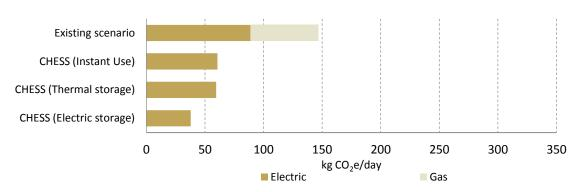
Figure 14. Dwellings totals equivalent CO2 emissions in the existing scenario and each CHESS Setup configurations
