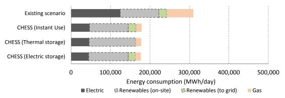
Figure 109. Dwellings totals energy uses/consumption in the existing scenario and each CHESS Setup configurations
