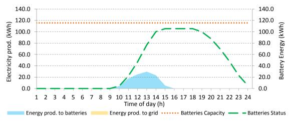
Figure 3. PVs electric production usage and batteries status.
