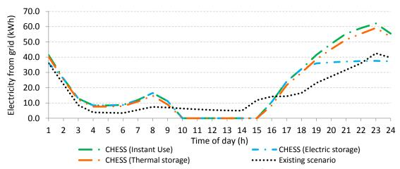
Figure 2. Dwellings existing scenario and CHESS Setup configurations hourly electric grid consumption
