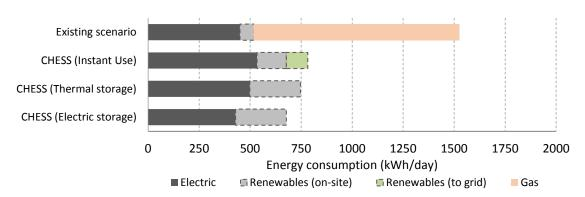
Figure 6. Dwellings totals energy uses/consumption in the existing scenario and each CHESS Setup configurations
