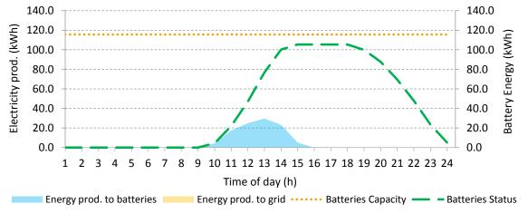
Figure 11. PVs electric production usage and batteries status
