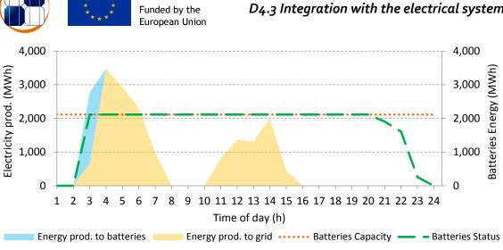
Figure 97. PVs electric production usage and batteries status.
