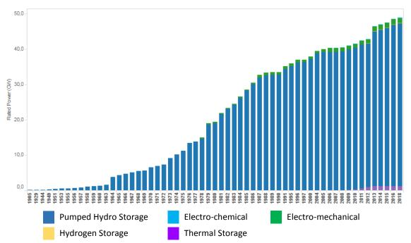
Figure 5. EU-28 Energy Storage Project Installations Over Time, adaptation of DOE database (DOE, Office of Electricity Delivery & Energy, 2016)
