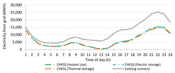
Figure 101. Dwellings existing scenario and CHESS Setup configurations hourly electric grid consumption
