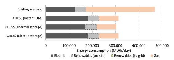
Figure 71. Dwellings totals energy uses/consumption in the existing scenario and each CHESS Setup configurations
