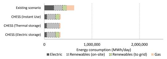
Figure 55. Dwellings totals energy uses/consumption in the existing scenario and each CHESS Setup configurations
