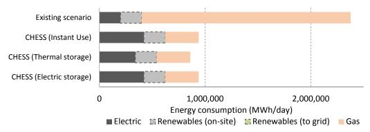
Figure 50. Dwellings totals energy uses/consumption in the existing scenario and each CHESS Setup configurations
