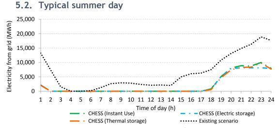
Figure 52. Dwellings existing scenario and CHESS Setup configurations hourly electric grid consumption
