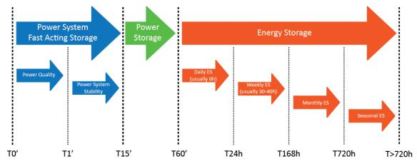
Figure 7. Energy storage applications segmented by discharge time (EASE/EERA Core Working Group, 2017)
