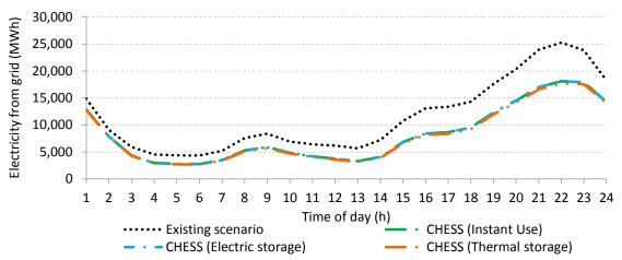
Figure 81. Dwellings existing scenario and CHESS Setup configurations hourly electric grid consumption
