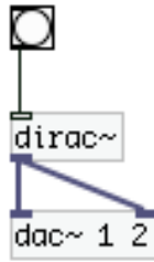
Figure 1.16.: The [dirac~] object produces an impulse if we send it a bang.
