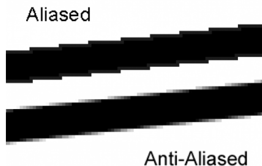
Figure 1.8.: Spatial aliasing in graphics. The “frequency” of the intended pixels is too high for the actual pixels.
