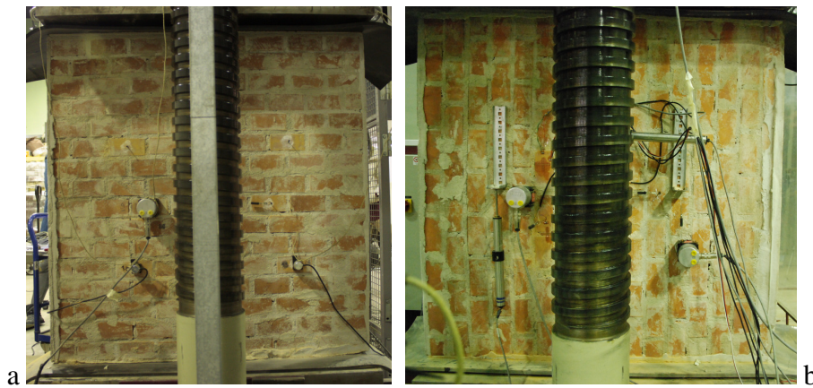
Figure 2: Compressive tests on masonry panels. Laboratory test configuration for compression normal to bed joints (a) and parallel to bed joints (b).
