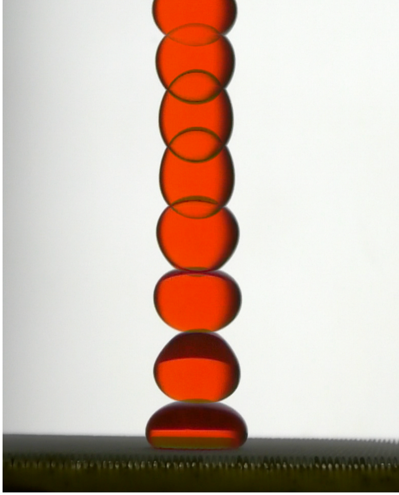
Figure 1.1: The trajectory of a 0.2 mL spontaneous drop jump is captured in a composite image over a period \sim 0.67 s presented at \approx 10 Hz.
