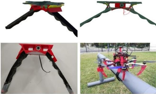
Fig. 2: From left to right bottom: CAD design of the soft gripper landing system; CAD design middle cut; Complete land gear support; Complete aerial platform.
