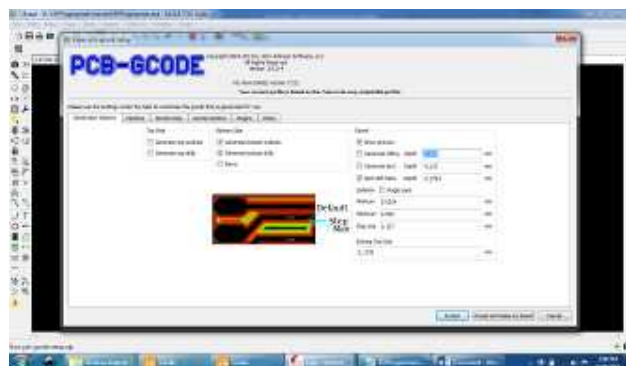
Fig.8: Converting PCB layout to G-code
