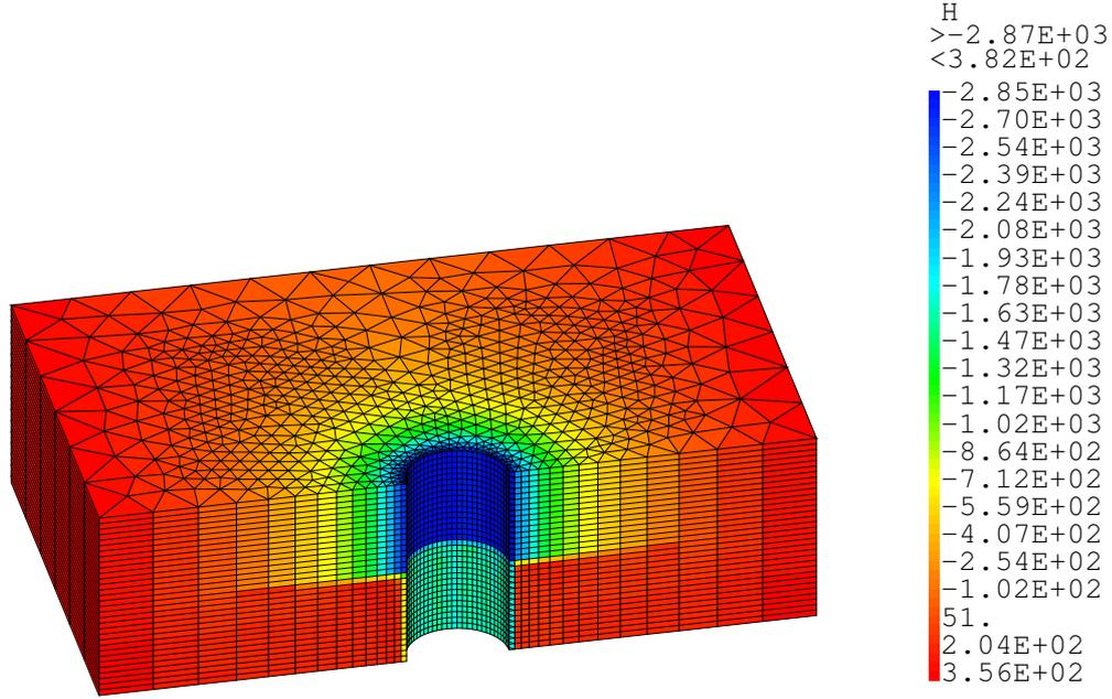
FIGURE 2. Pressure head inside the system at time  $t = 100 \text{ years}$ .
