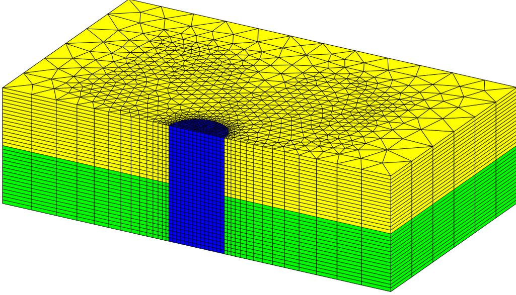
FIGURE 1. Mesh of the domain (40000 cells) constituted of host rock (green), permeable layer (yellow) and seal (blue).
