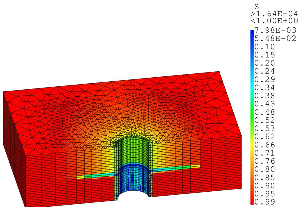
FIGURE 3. Saturation inside the system at time  $t = 100$  years.
