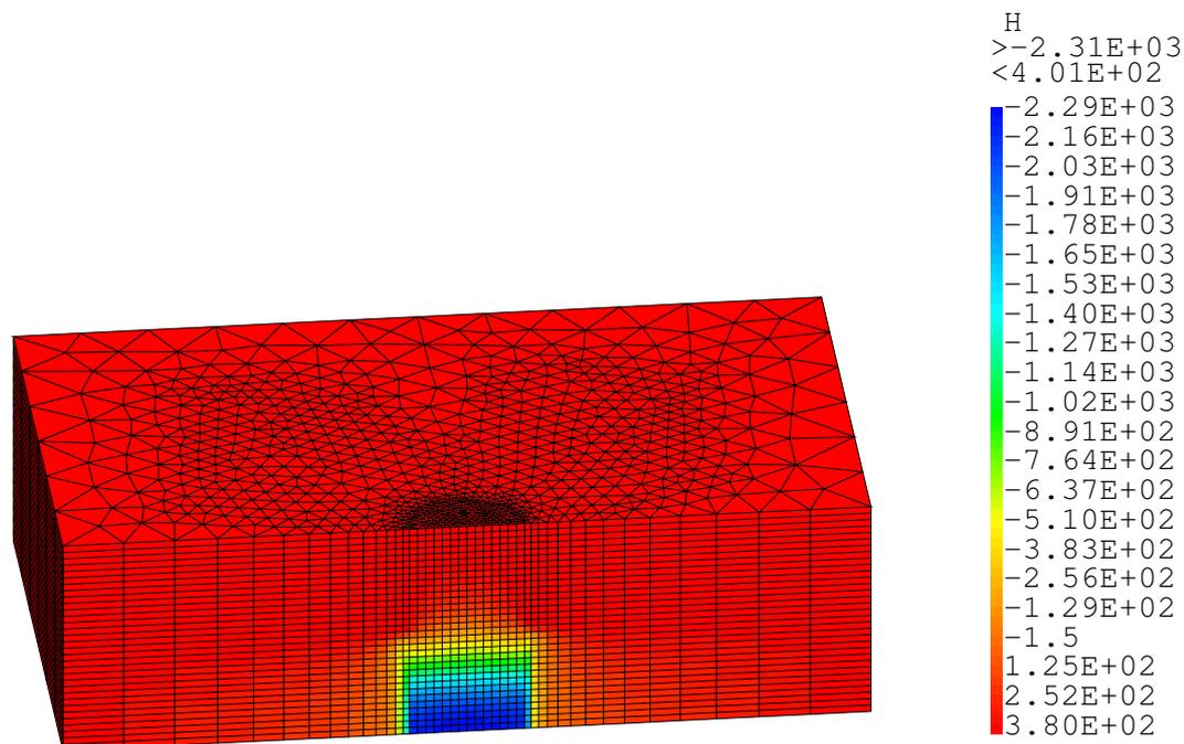
FIGURE 5. Pressure head inside the system at time  $t = 50$  years after closure.
