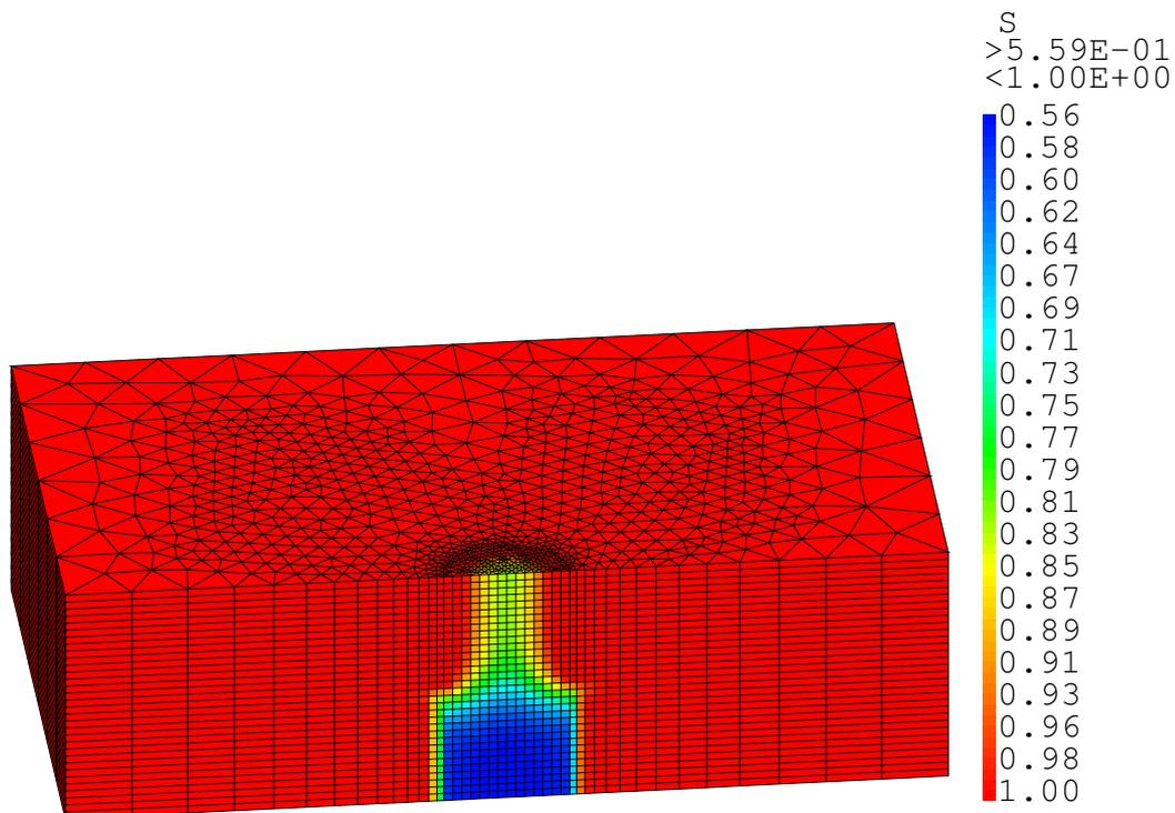
FIGURE 6. Saturation inside the system at time  $t = 15$  years after closure.
