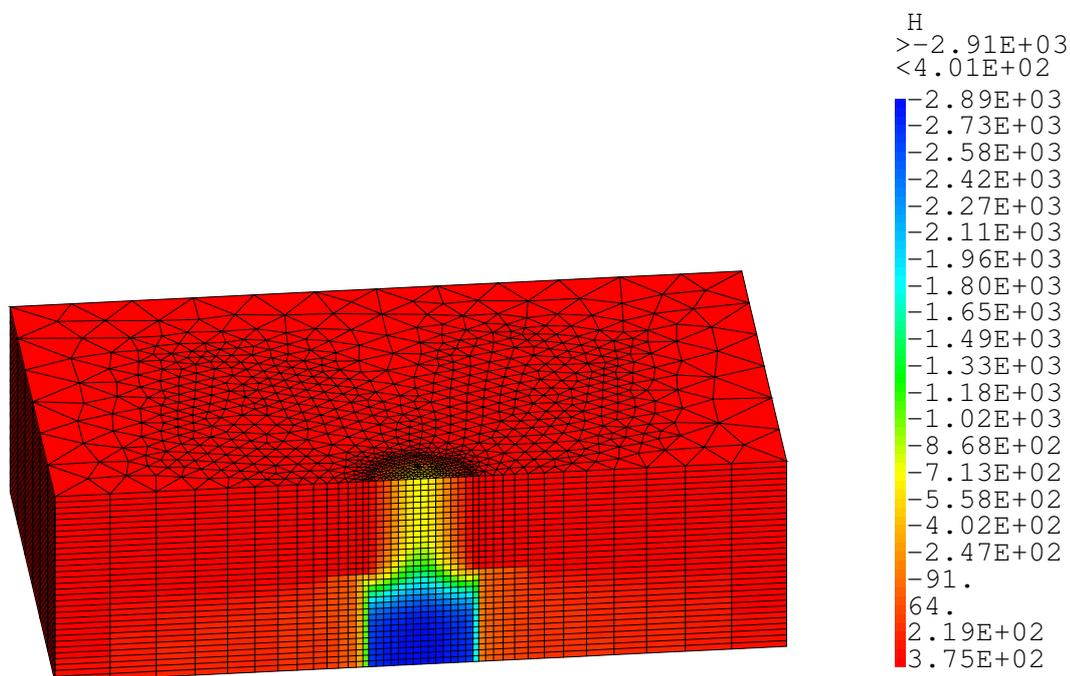
FIGURE 4. Pressure head inside the system at time  $t = 15$  years after closure.
