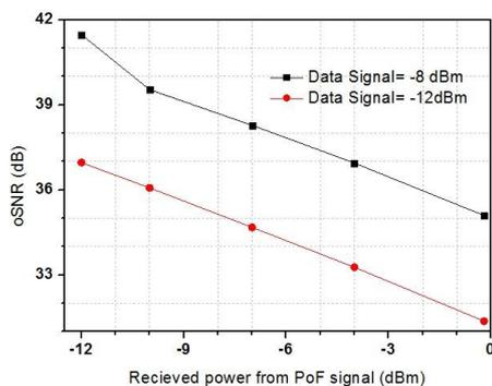
Fig. 2: Data signal oSNR at different power levels vs PoF power delivered at reception stage.
