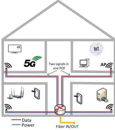
Fig. 1 Illustrative POF network for multi-standards wired and wireless transmission in the home applications with remote power delivery.
