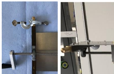
Figure 3: Connect the adjustable clamps to the stretching device (A) and to the standing supports (B)
