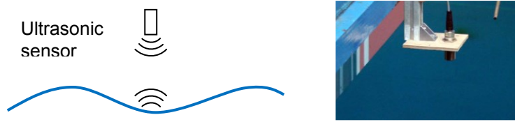
Figure 3.16 Ultrasonic wave gauge functional diagram and example at Ifremer
