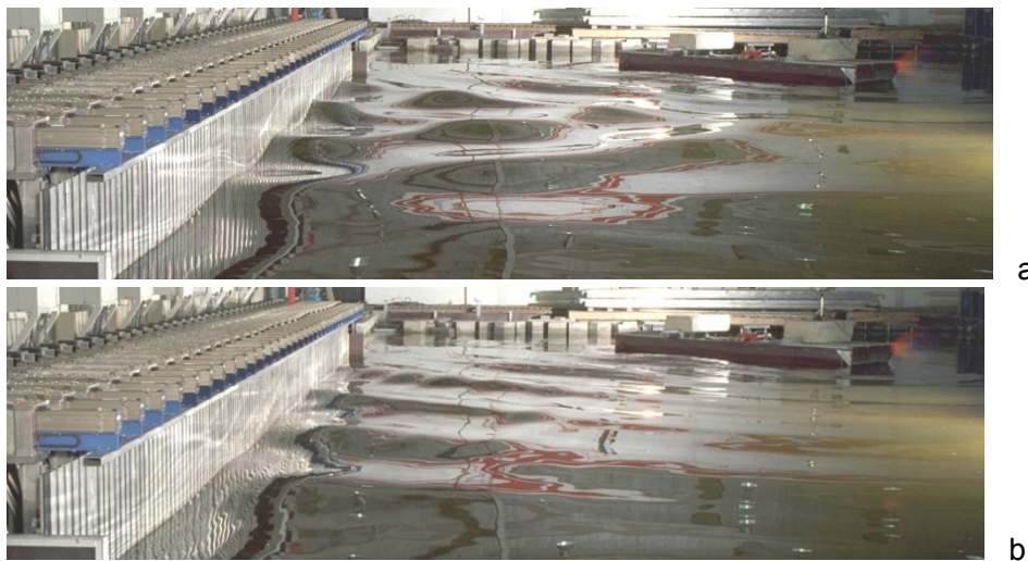
Figure 3.2 Oblique waves generated by the wave generator to the right. (a) 3D wavemaker at rest. (b) 3D wavemaker in absorbing mode.
