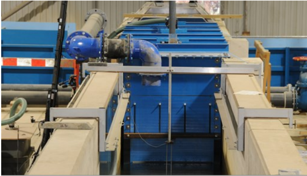
Figure 3.9 Tsunami Generator mounted within the wave flume, the adjustable outlet is in the foreground under water
