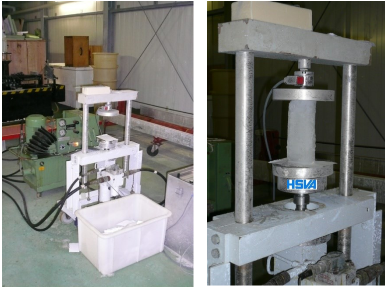
Figure 3.31 10 kN uni-axial compression testing machine as used at HSVA
