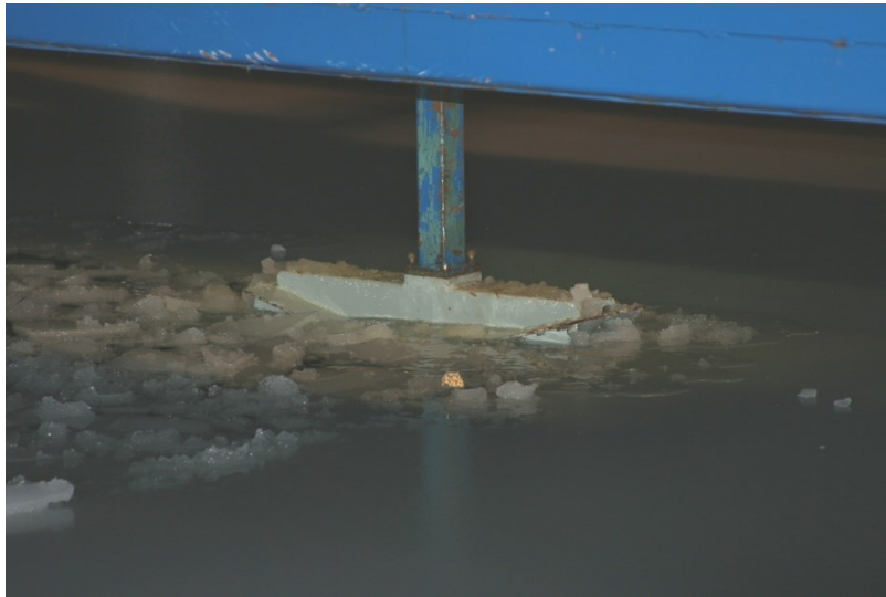
Figure 3.38 Production of a brash ice channel at Aalto University
