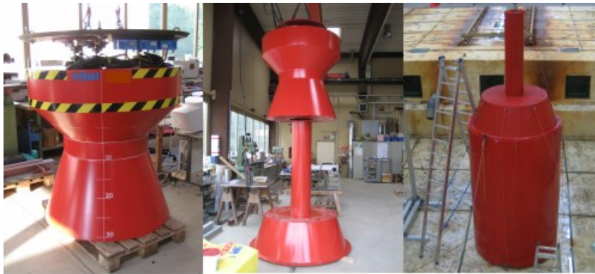
Figure 2.21 Different segments of the SPAR model (Evers & Jochmann, 2011)
