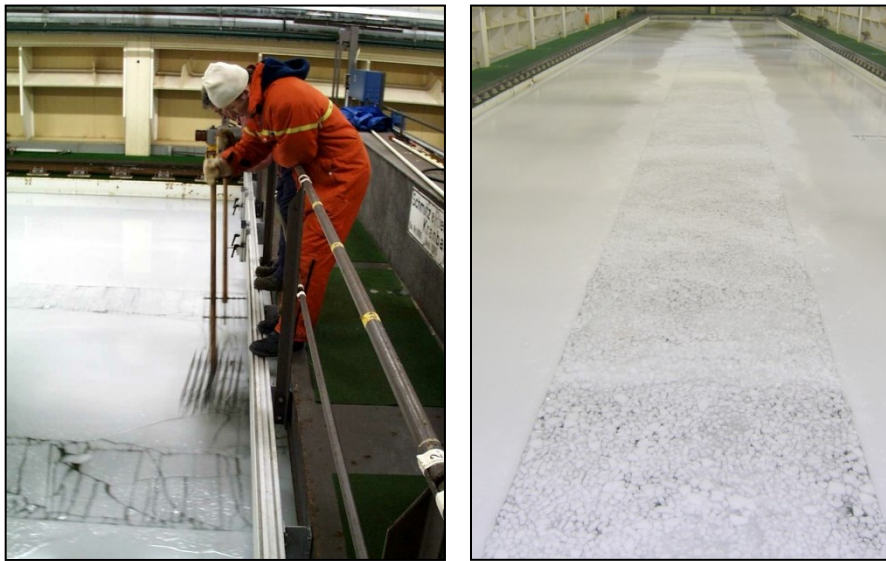
Figure 3.37 Preparation of brash ice channel at HSVA
