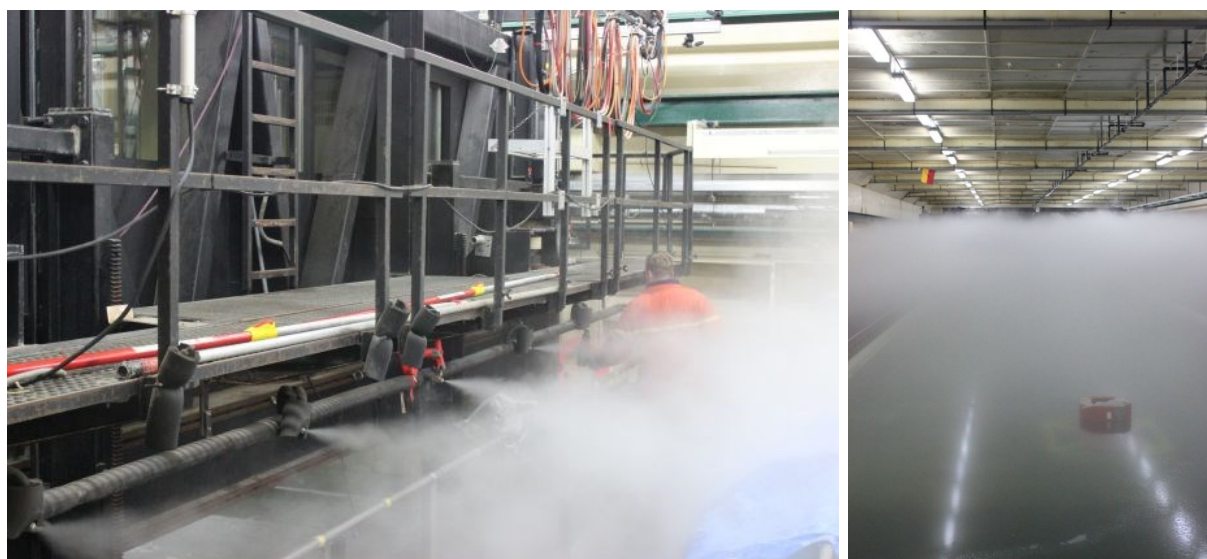
Figure 3.23 Water is sprayed under high pressure into the air of the pre-cooled ice tank at HSVA forming crystal nuclids which settle down on the water surface
