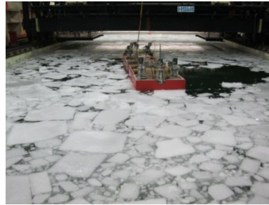
Figure 4.16 Digital photographs used to determine ice flow concentration and movement of elements
