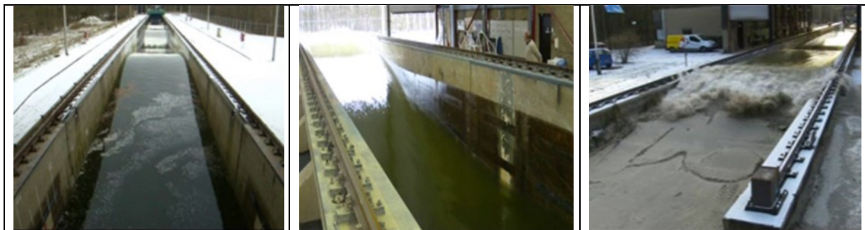
Figure 3.7 N-wave generated in old Delta Flume and overtopping a dike slope (Hofland et al 2013)
