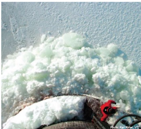
Ice crushing failure at Lighthouse Norströmsgrund, Sweden (Photo: K. Kolari, VTT)
