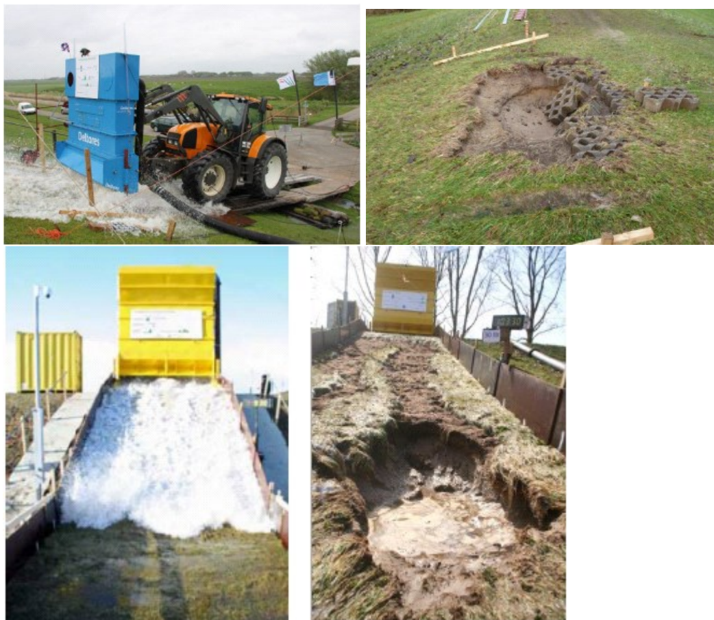
Figure 7.1 Pictures of process simulators. Top left: wave impact generator with erosion generated (top right). Bottom left: wave impact generator at sand dike with erosion generated (bottom right)
