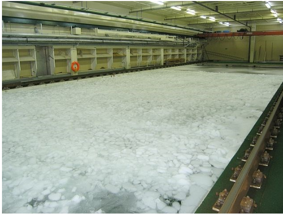
Figure 3.51 Ice rubble field at HSVA's ice tank (left), moored FPU model entering the ice rubble astern (right)
