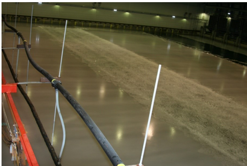
Figure 3.39 Brash ice channel (Aalto University)
