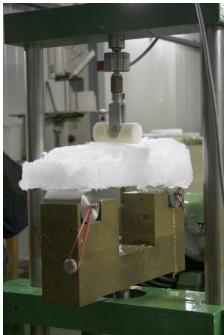
Figure 3.29 3-point loading beam (downward loading)
