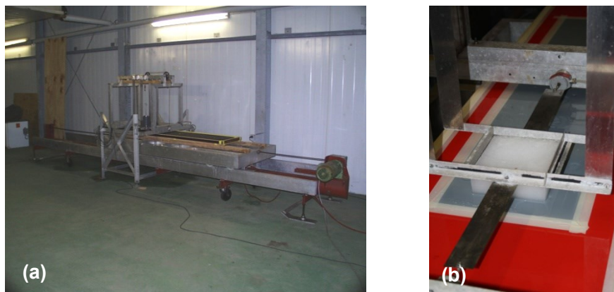
Figure 4.5 (a) Friction testing device; (b) ice sample loaded between load cells
