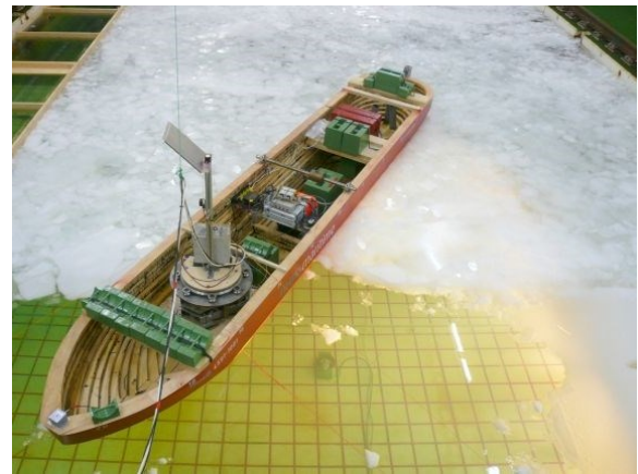
Figure 3.51 Ice rubble field at HSVA's ice tank (left), moored FPU model entering the ice rubble astern (right)
