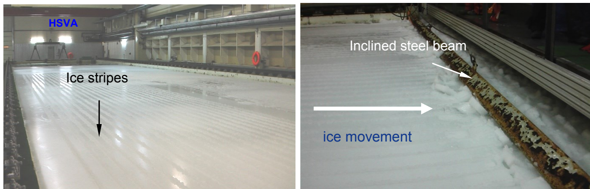
Figure 3.40 Ice sheet cut into stripes (left) and steel beam submerging ice when pushed by towing carriage (right)
