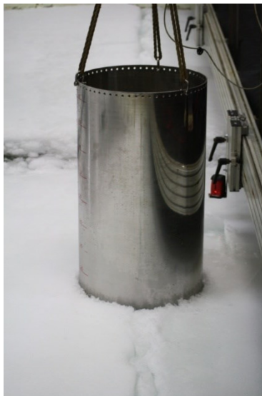
Figure 3.47 Test set-up of the punch tests
