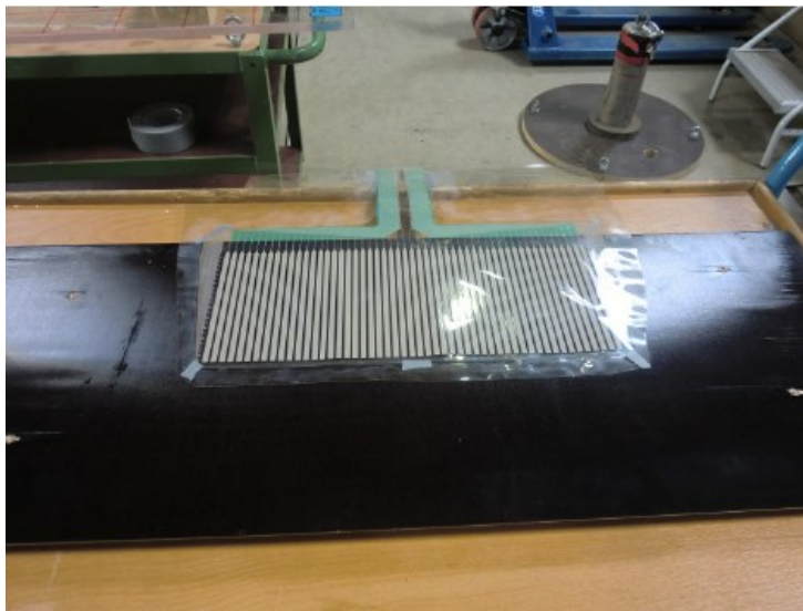
Figure 6.11 Waterproof protection by plastic films
