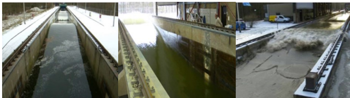
Figure 6.3 N-wave generated in old Delta Flume travelling through flume and overtopping a dike slope (Holland et al 2013)
