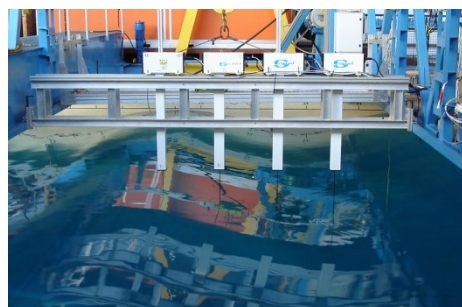
Figure 3.15 Servo wave gauge functional diagram and example at Ifremer
