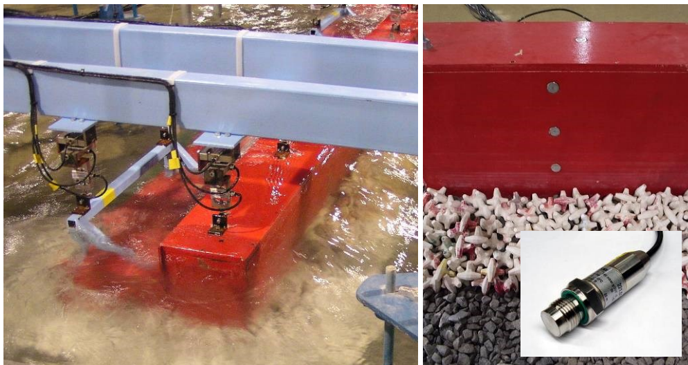
Figure 4.8 Caisson with rigid force measurement rig (left) and pressure sensors (right)
