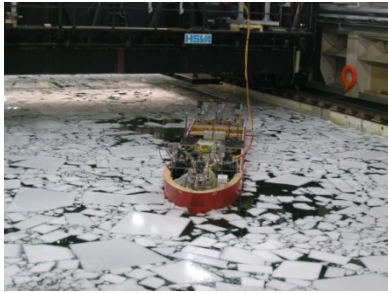
Figure 4.16 Digital photographs used to determine ice flow concentration and movement of elements
