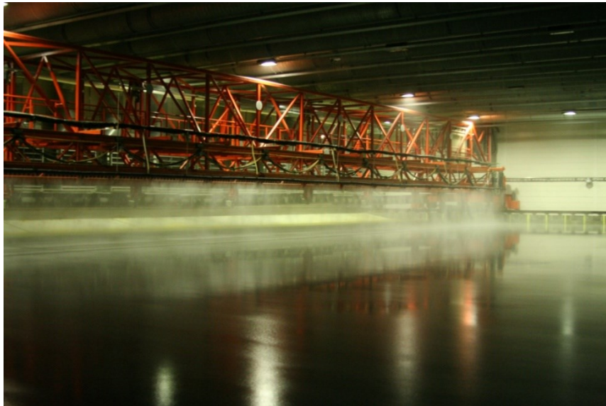
Figure 3.25 The spraying process at Aalto University
