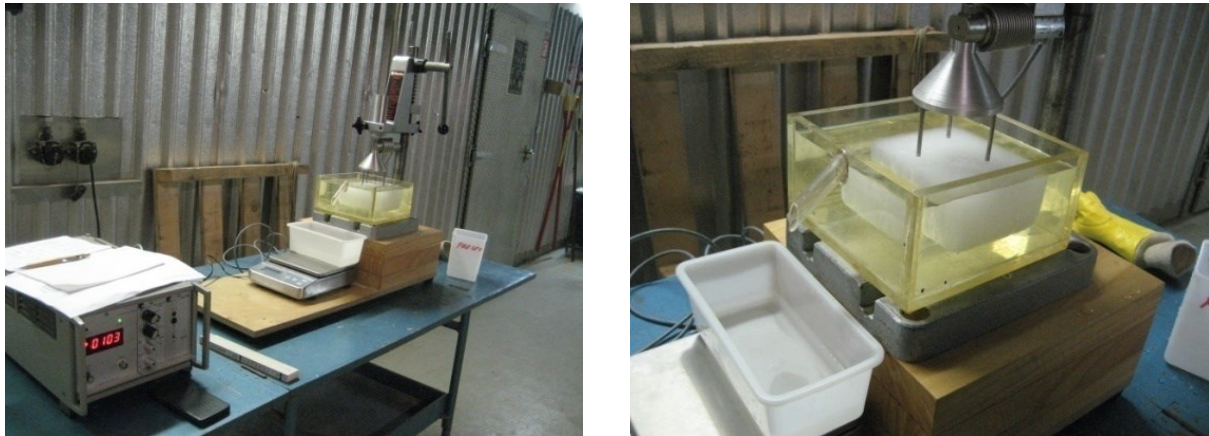
Figure 3.32 Test setup for ice density tests at HSVA
