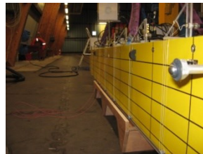
Figure 3.14 Capacitive wave gauge functional diagram and example of set up on a model at Ifremer
