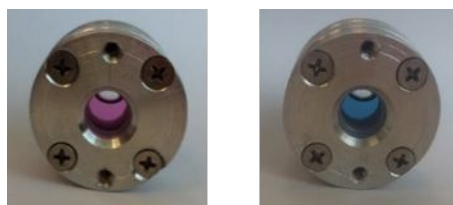
Fig. 2 Aqueous MEG-PBI solutions at RT (left) and 313 K (right).
