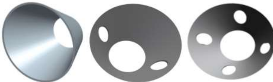
Fig. 2. Schematic view of perforated conical rings with N= 0, 2, 4 respectively.
