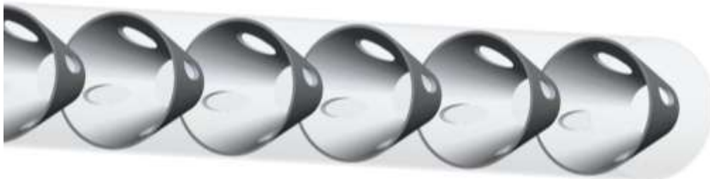
Fig. 3. Schematic view of tube assembly with inserts with N= 4 & PR=1 .
